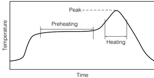
For soldering (Example : Sn/Pb)
