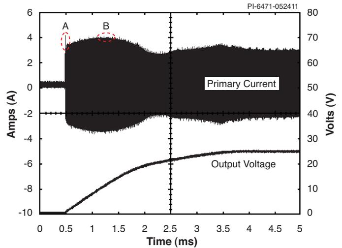
Figure 22. Typical Start-up Waveform. Observe Initial Current Spike 'A' to Ensure it is Below the 1-Cycle Current Limit. A Higher  $f_{MAX}$  Reduces it. Size the Soft-Start Capacitor so that the Peak of 'B' is just Below the Peak Current at  $V_{BROWNOUT}$  at Full Load.
