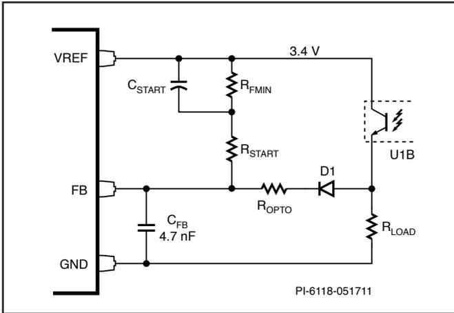
Figure 19. Feedback Network Shown with Additional Load Resistor.
