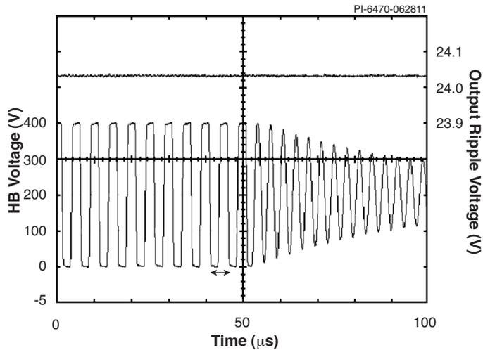
Figure 26. Zoom in of Last Few Switching Cycles of Burst Pulse Train of Figure 24. The Switching Frequency of the Last Few Cycles is  $f_{STOP}$  383 kHz in This Case (arrow). The Ringing in  $V_{HB}$  After Switching Stops, is the Primary Inductance Ringing with the MOSFET Capacitance.
