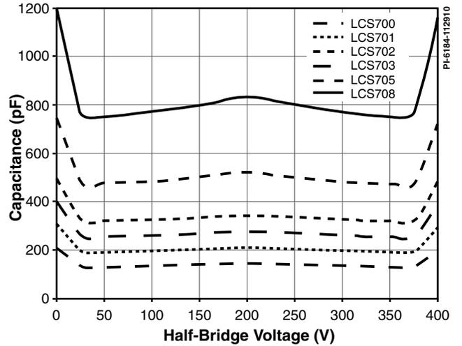
Figure 30. Half-Bridge Small Signal Capacitance vs. Half-Bridge Voltage.
