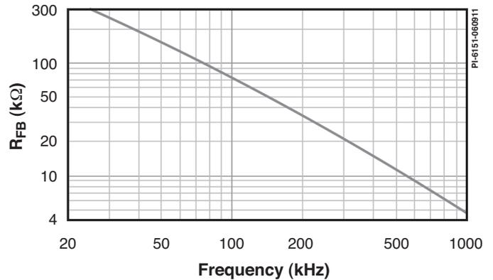
Figure 21. VREF to FB External Resistance vs. Frequency.
