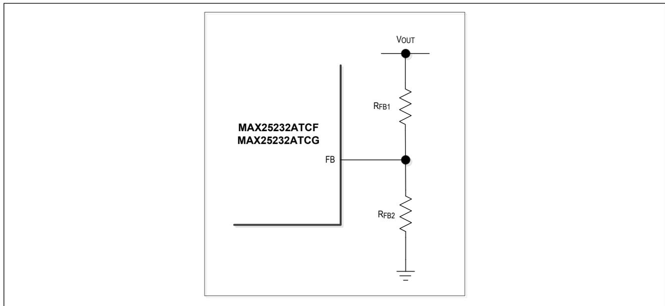
Figure 1. Setting the Output Voltage with External Resistor-Dividers
