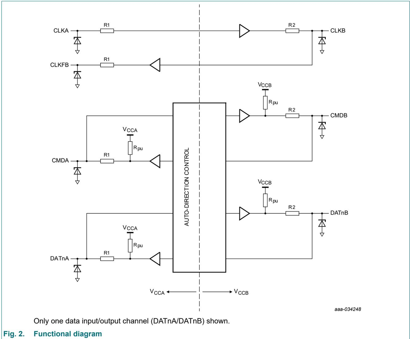
**Fig. 2. Functional diagram**
