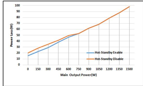
Figure 8. PSU power losses with/without hot-standby mode
