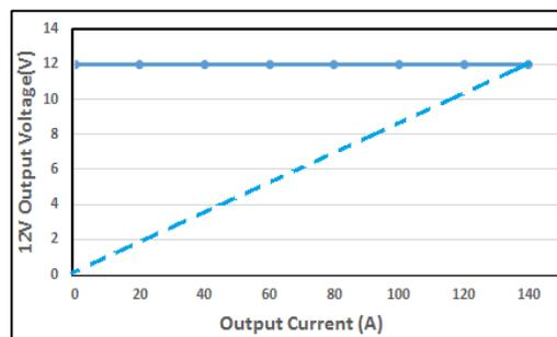
Figure 6. Current Limitation on  $V_1$  ( $V_1 = 230\text{ VAC}$ )
