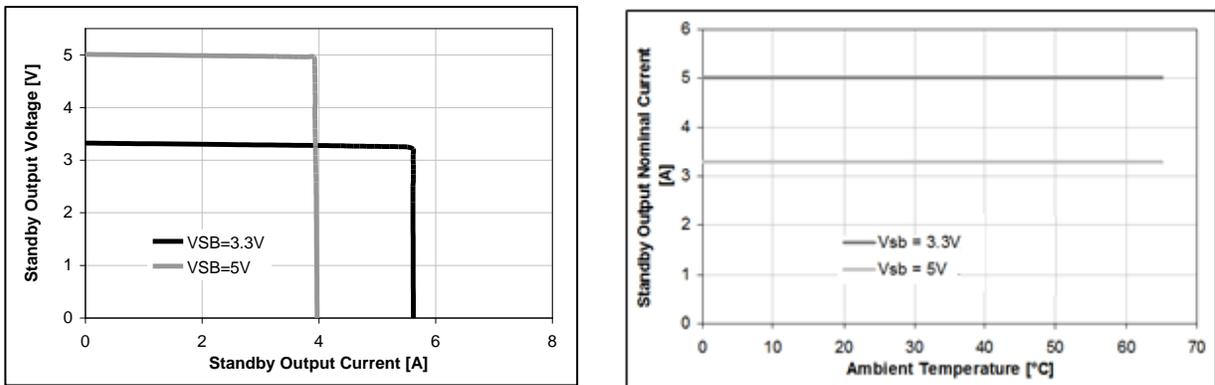
Figure 8. Current Limitation and Temperature Derating on 3.3 / 5 V<sub>SB</sub>
