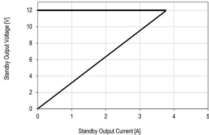
Figure 9. Current Limitation on 12 V<sub>SB</sub>
