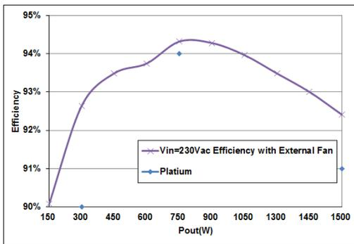
Figure 2. Efficiency vs. Load current (ratio metric loading)
