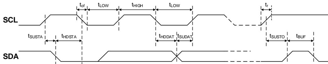
Figure 20. I2C / SMBus Timing
