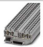
Component terminal block, Connection method: Spring-cage connection, Cross section: 0.08 mm² - 4 mm², AWG: 28 - 12, Width: 5.2 mm, Color: gray, Mounting type: NS 35/7,5, NS 35/15
