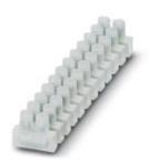
Polyamide Europe terminal strip, transparent, with wire protection, for connecting solid conductors and stranded conductors with and without ferrules with a cross section of 0.75 to 4 mm²
