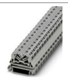
Mini feed-through terminal block, Connection method: Spring-cage connection, Cross section: 0.08 mm² - 4 mm², AWG: 28 - 12, Width: 10.4 mm, Height: 22 mm, Color: blue, Mounting type: NS 35/7,5, NS 35/15
