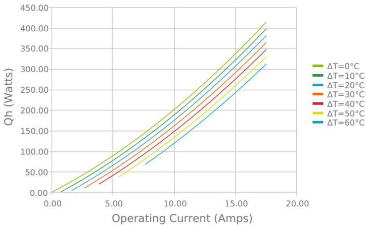
Total Heat Dissipated at Hot Side (Qh=Qc+Pin)
