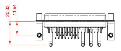
**OPERATING TEMPERATURE:** -55°C ~ 125°C POWER/CO-AX CONTACT RATING: 20A (CURRENT) (IF PRESENT) SIGNAL CONTACT CURRENT RATING: 5A PER CONTACT SIGNAL CONTACT RESISTANCE:  $10m\Omega$  MAX.
