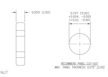
ΝΠΤΕ: MATERIAL HOUSING: PBT UL94V-0, BLACK CONTACT: BRASS NUT: BRASS SHELL: BRASS □-RING: NBR, BLACK FINISH GOLD PLATED CONTACT: OVER 504" NICKEL NUT: NICKEL PLATED NICKEL PLATED SHELL: ELECTRICAL RATED CURRENT: 1A RATED VOLTAGE: 60V INSULATION RESISTANCE: 100 MOhms MIN. CONTACT RESISTANCE: 10 mOhms MAX. WATER PROOF: IP67 **ENVIRONMENT** OPERATION TEMPERATURE: -40°C TD +85°C WIRE GAUGE: 28 AWG MAX RECOMMENDED
