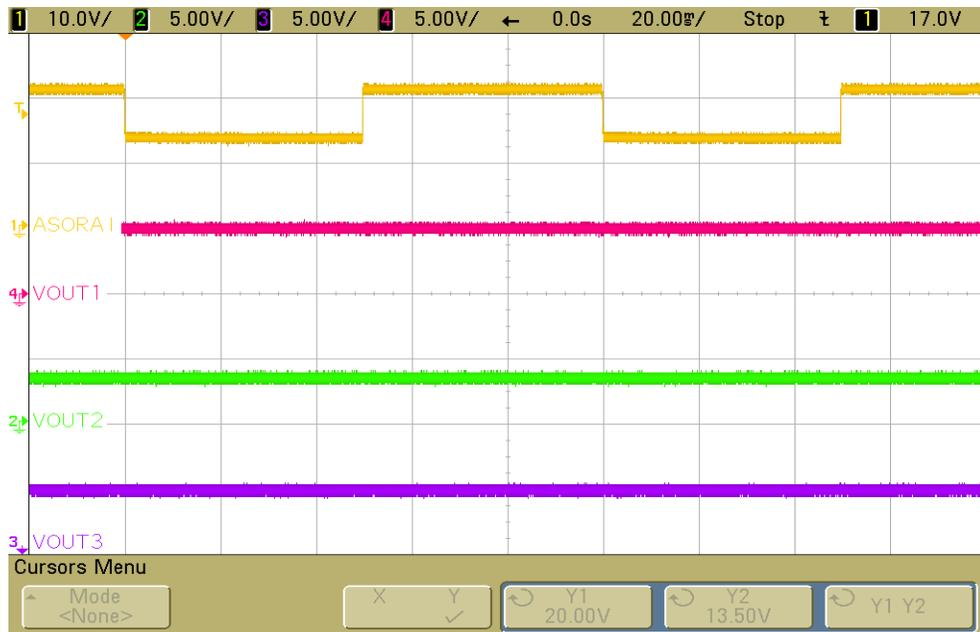
Figure 35. Output Response to OVS - VBAT-MON Left Open
