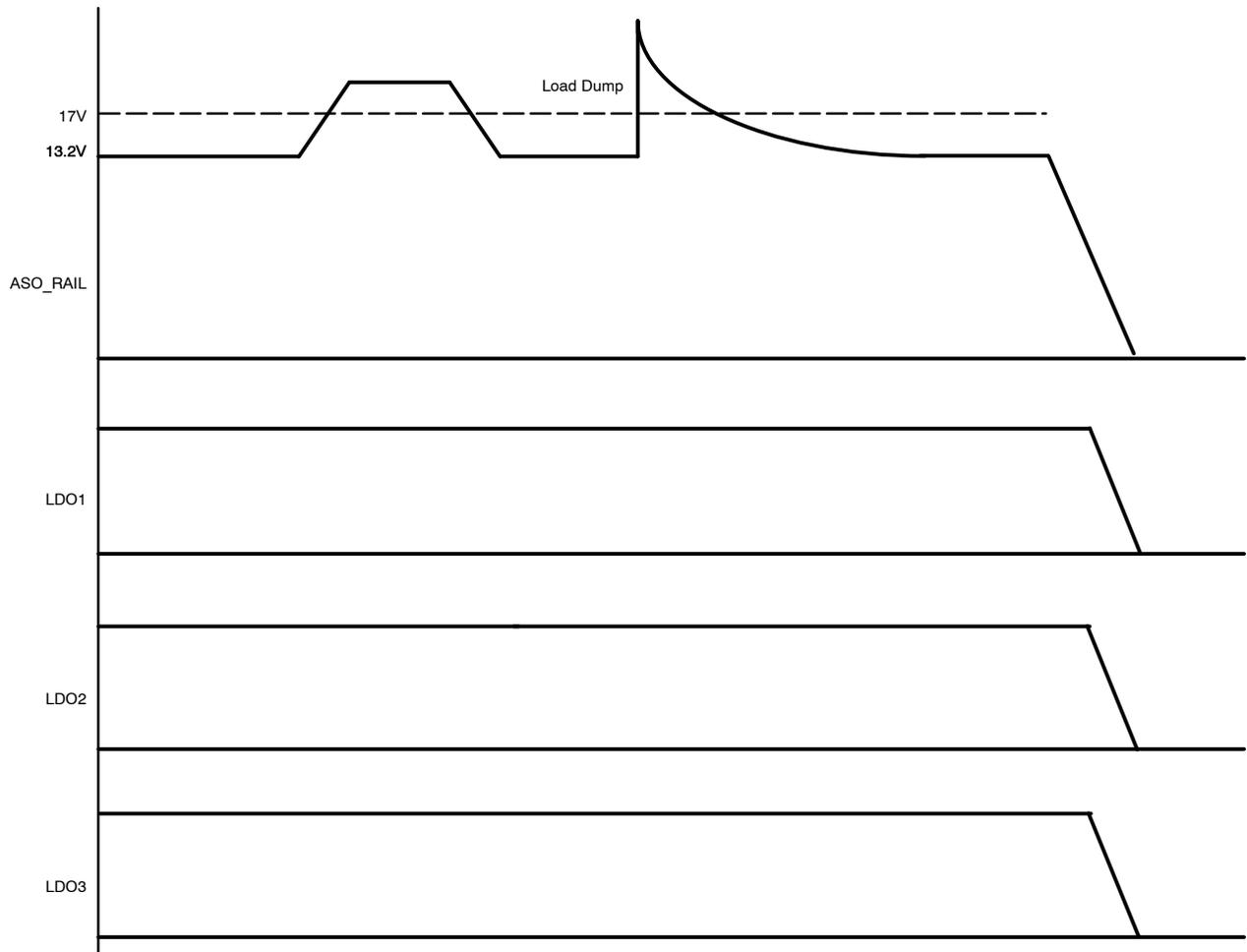
Figure 11. NCV8614B Regulator Output Timing Diagram- VBATT\_MON Grounded
