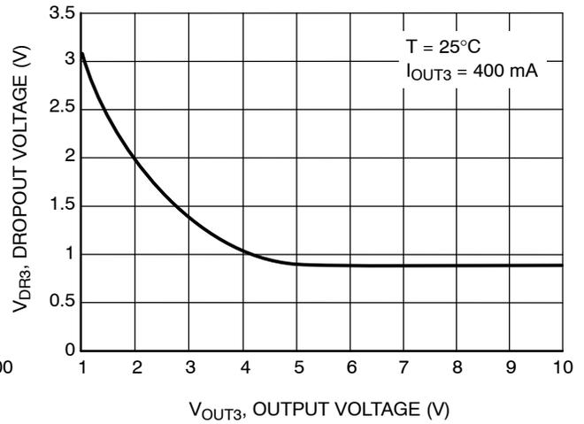
Figure 19. LDO3 Dropout Voltage vs. Output Voltage
