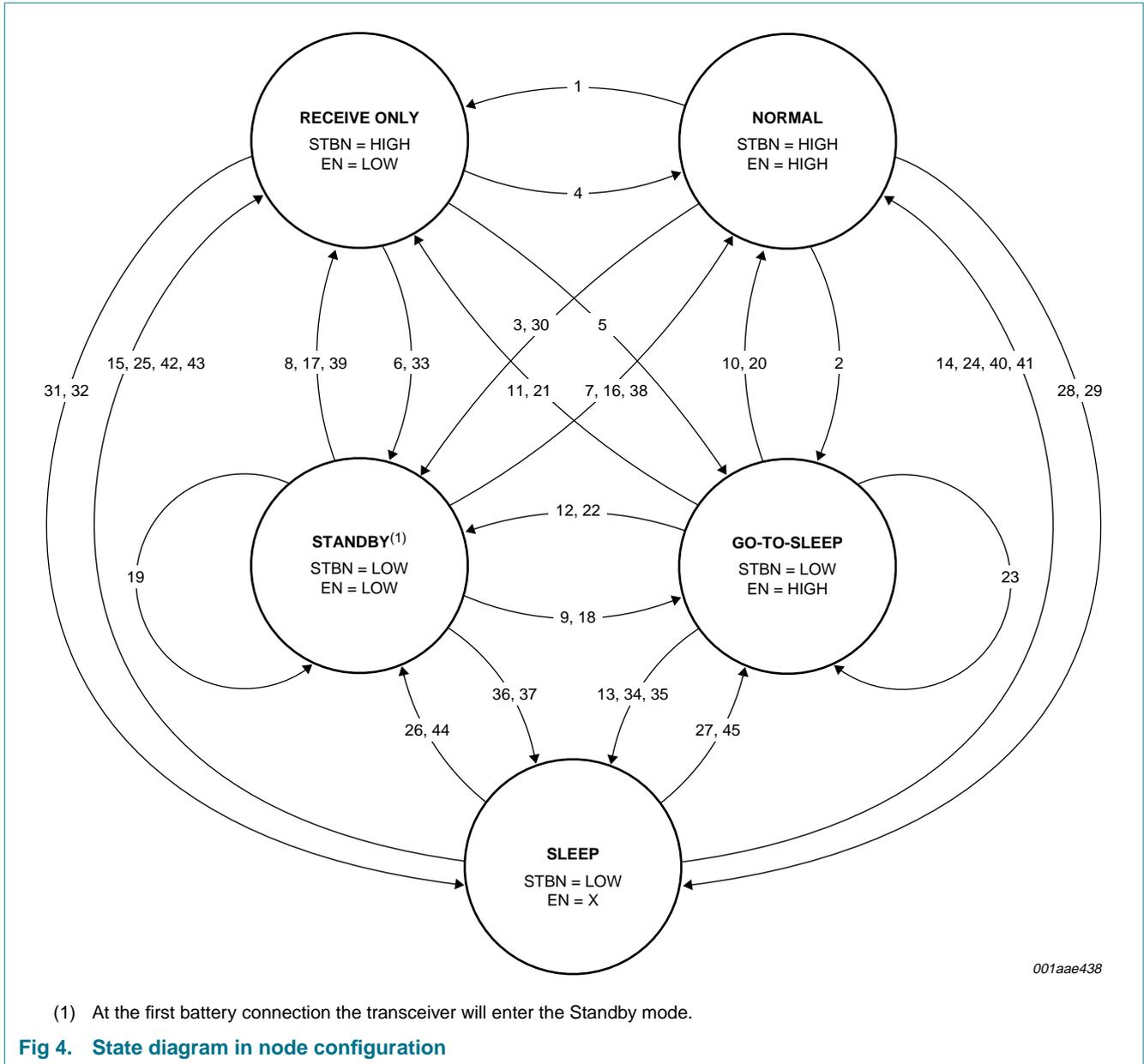
The state transitions are represented with numbers, which correspond with the numbers in the last column of [Table 5](#) to [Table 8](#).
