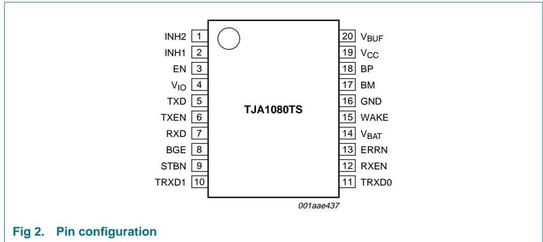
Fig 2. Pin configuration
