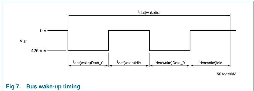
Fig 7. Bus wake-up timing
