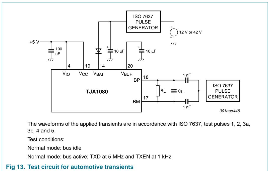
The waveforms of the applied transients are in accordance with ISO 7637, test pulses 1, 2, 3a, 3b, 4 and 5.
