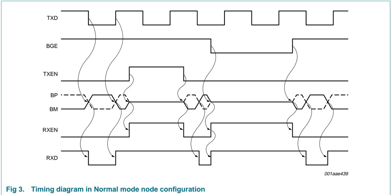
**Fig 3. Timing diagram in Normal mode node configuration**
