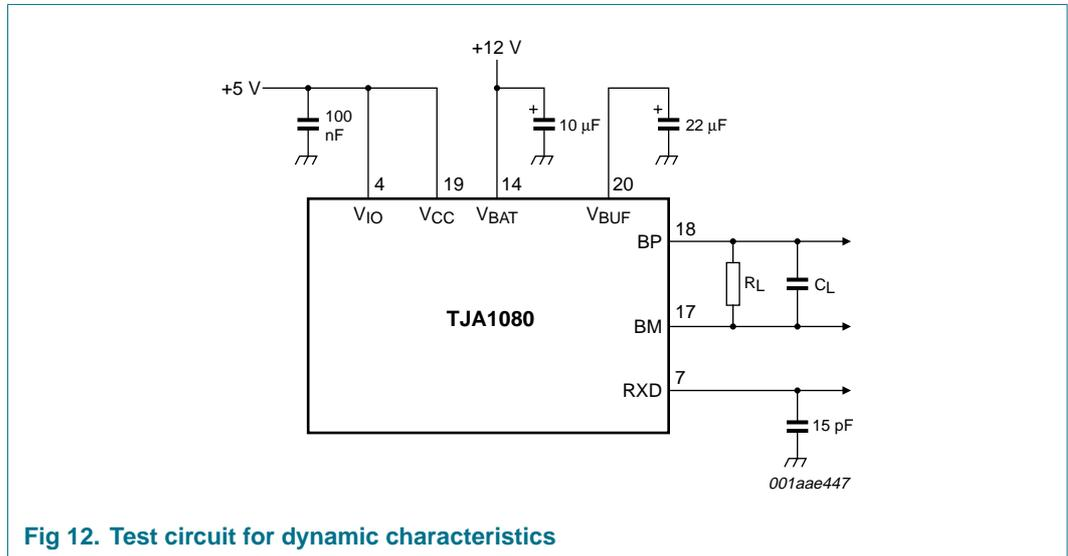
Fig 12. Test circuit for dynamic characteristics
