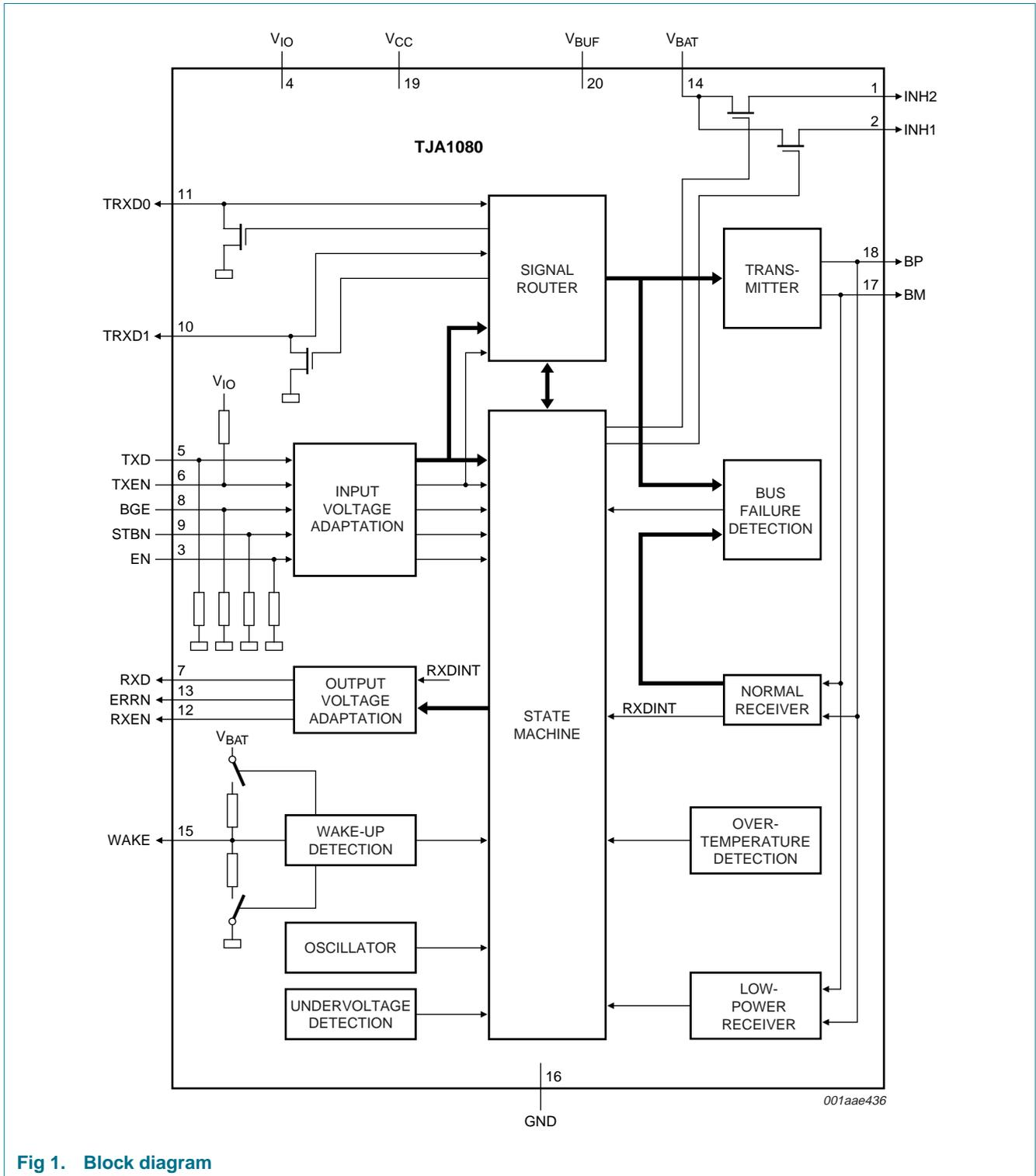
Fig 1. Block diagram
