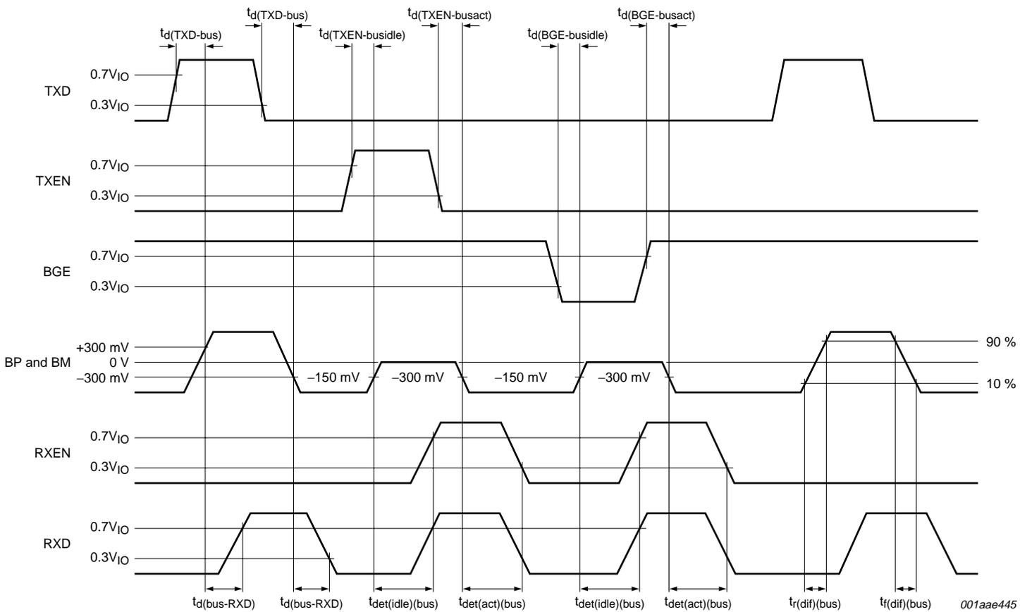
Fig 10. Detailed timing diagram in node configuration
