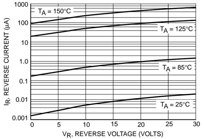
Figure 3. Leakage Current
