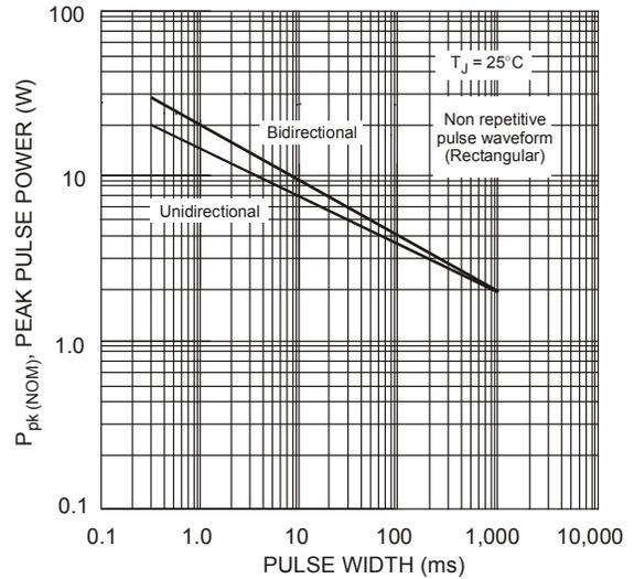
Fig. 6 Pulse Rating Curve,
