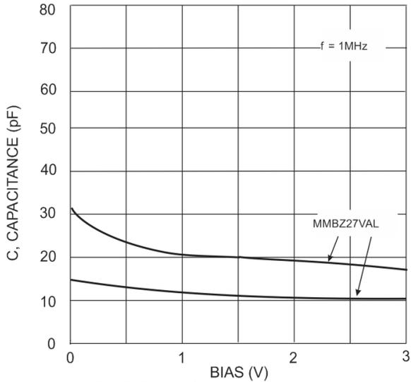
Fig. 3 Typical Capacitance vs. Bias Voltage
