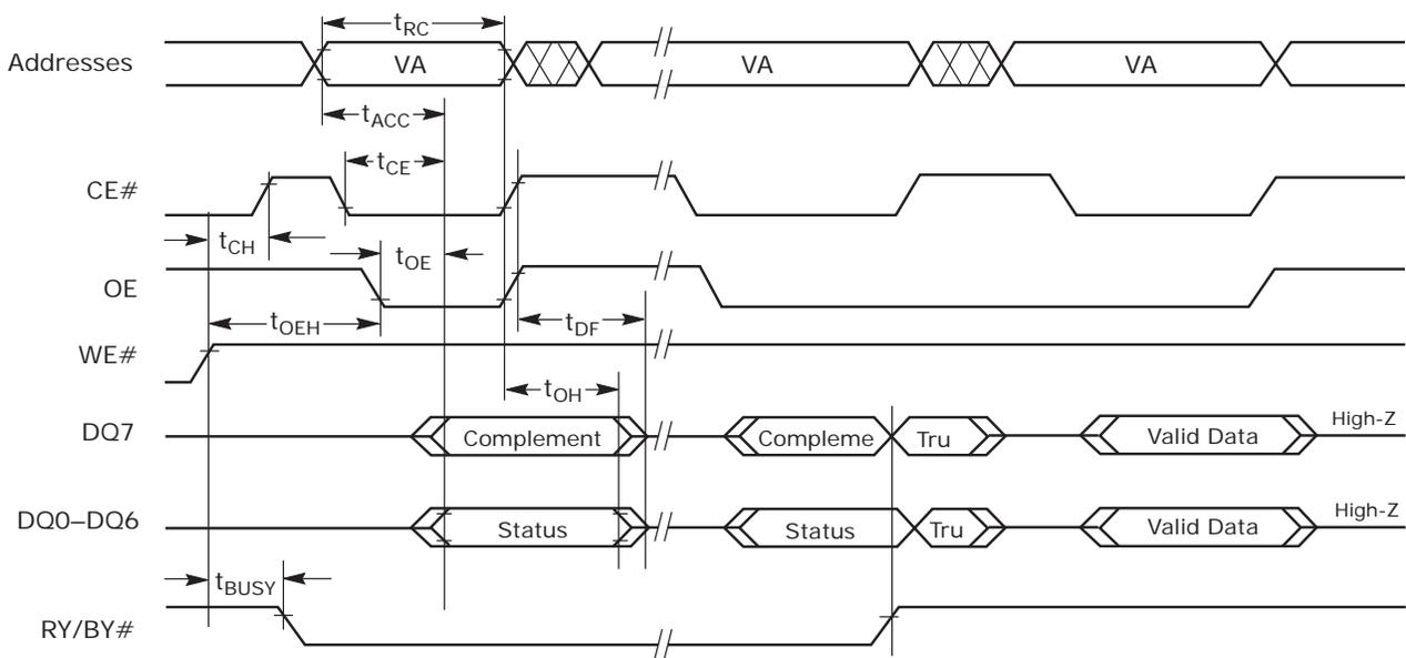
Figure 19. Toggle Bit Timings (During Embedded Algorithms)<sup>[58]</sup>
