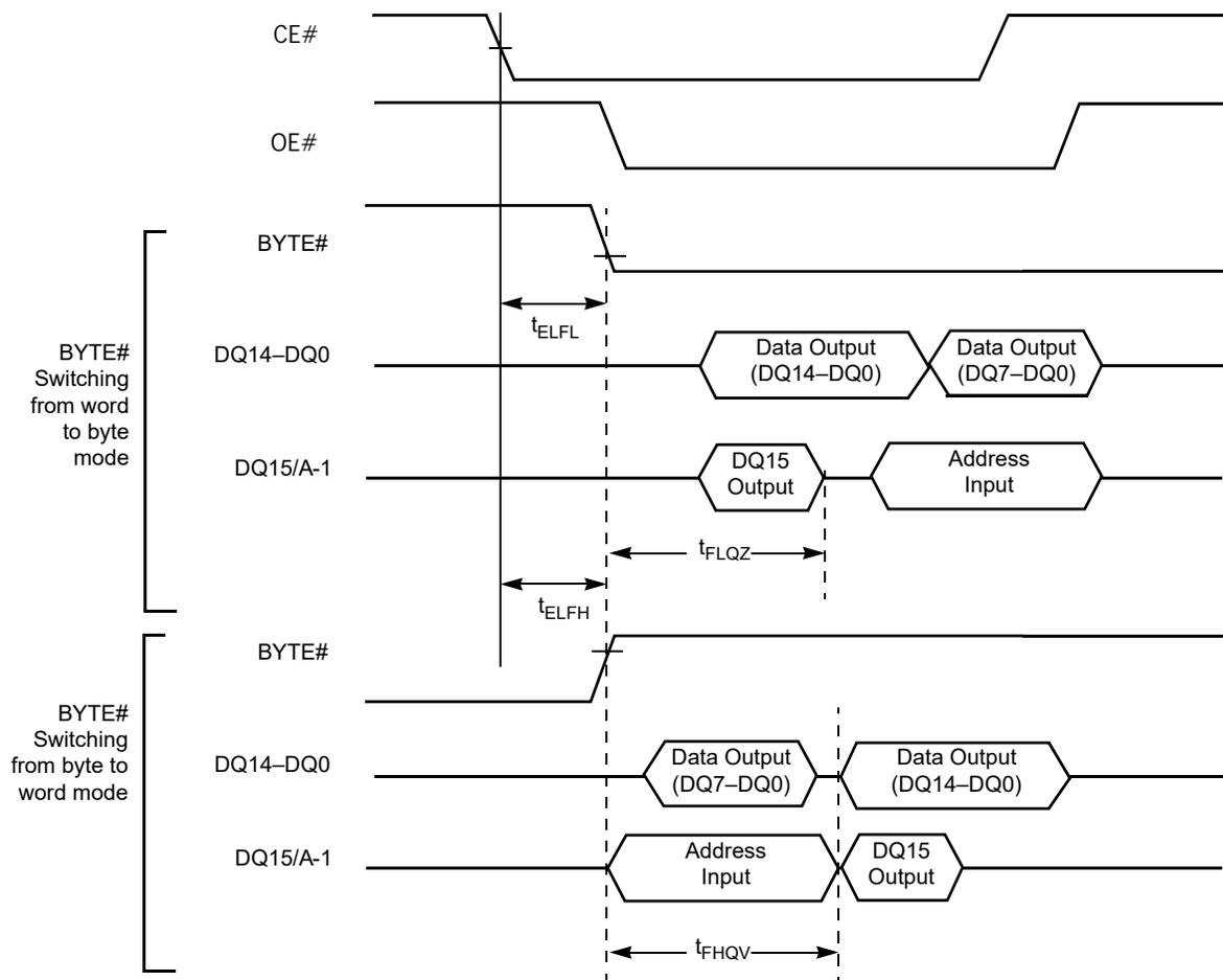
Figure 17.2 BYTE# Timings for Write Operations<sup>[50]</sup>
