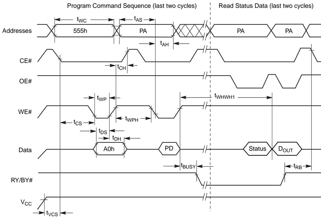
Figure 15. Accelerated Program Timing Diagram
