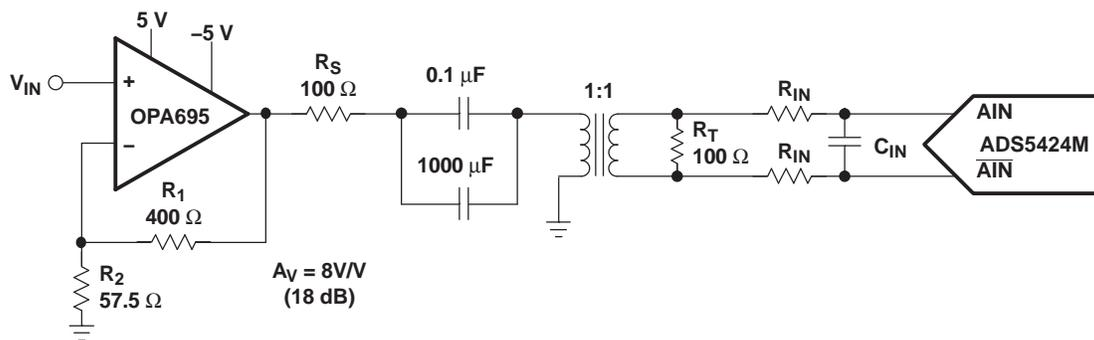
Figure 18. Using the OPA695 With the ADS5424
