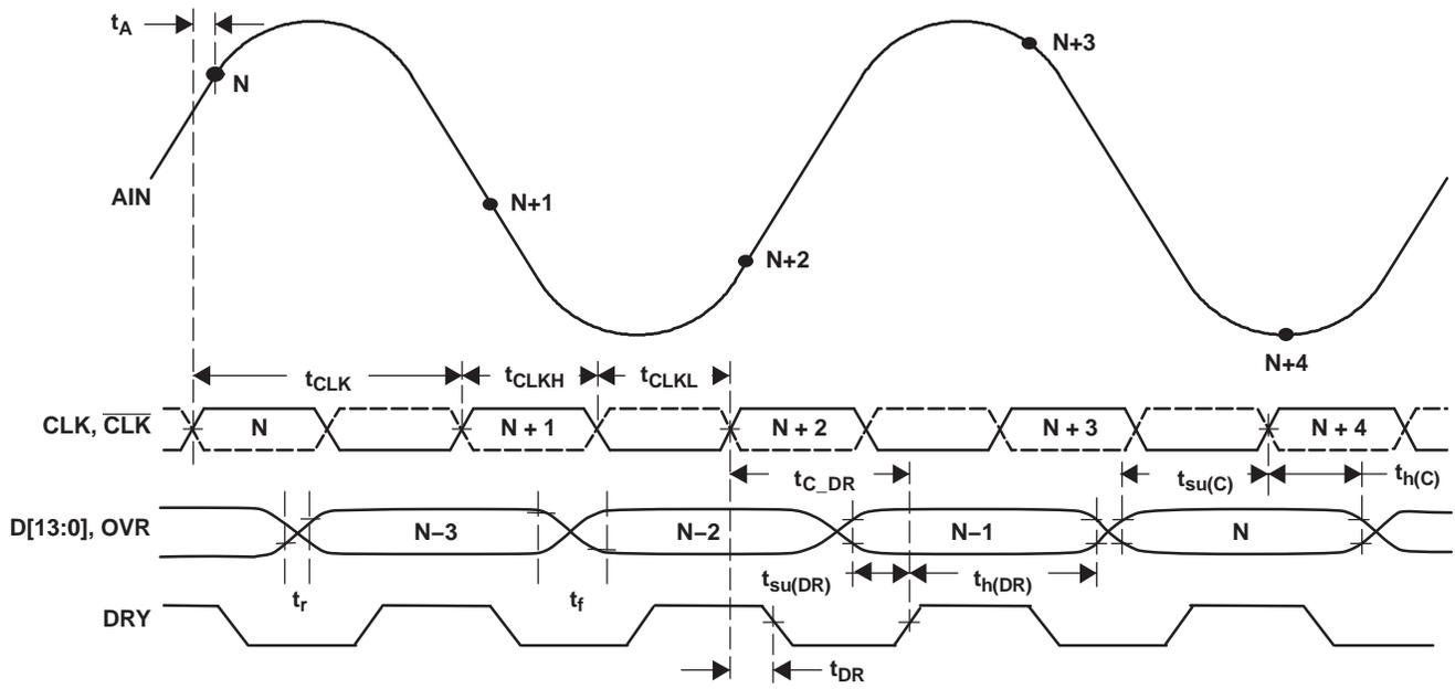
Figure 1. Timing Diagram
