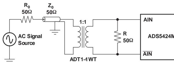
Figure 17. Converting a Single-Ended Input to a Differential Signal Using RF Transformers
