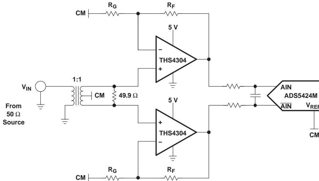
Figure 19. Using the THS4304 With the ADS5424
