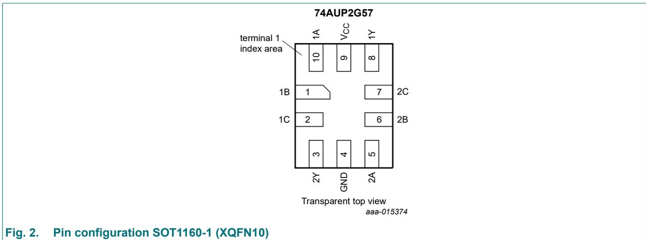
Fig. 2. Pin configuration SOT1160-1 (XQFN10)
