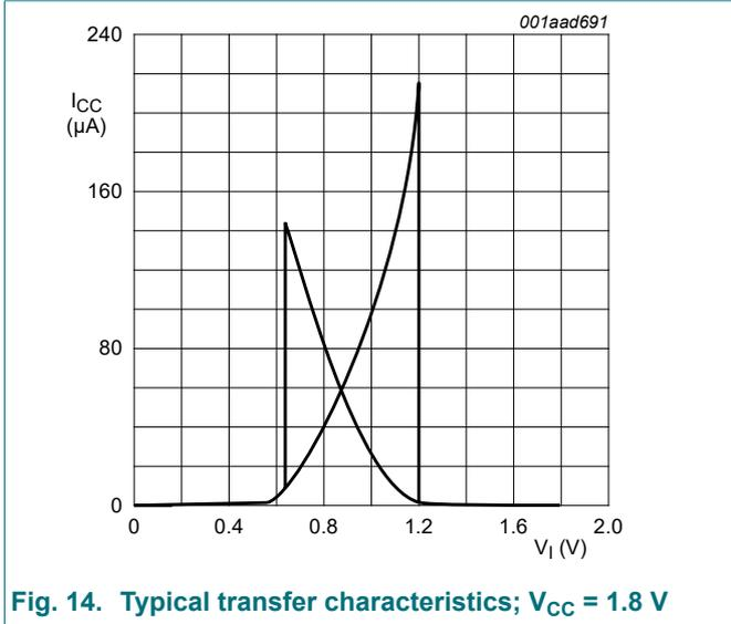
Fig. 14. Typical transfer characteristics;  $V_{CC} = 1.8 V$
