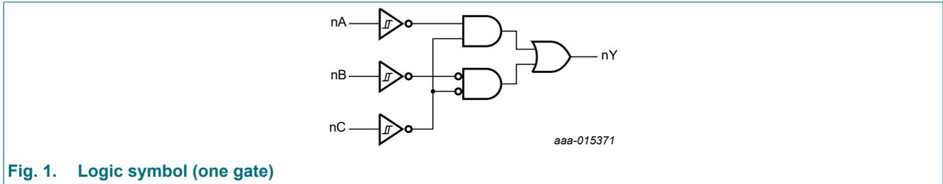
Fig. 1. Logic symbol (one gate)
