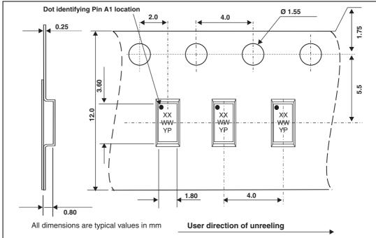
Figure 11. µQFN-16L tape and reel specification
