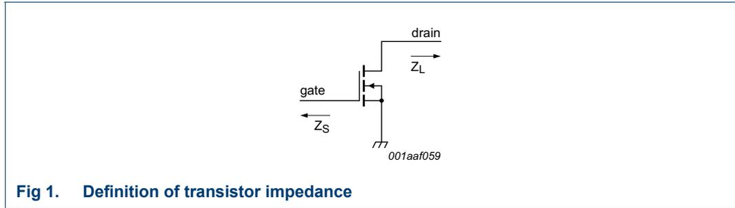
Fig 1. Definition of transistor impedance
