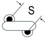
The measurement position of Lead Spacing (S) and Width (V) is critical in straight lead capacitors.
