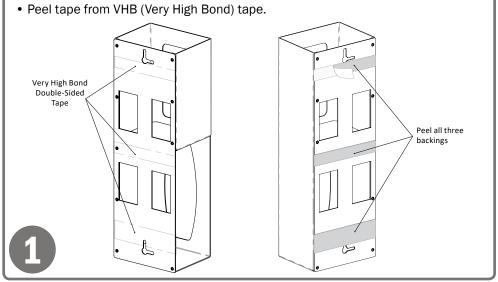
VHB tape is virtually permanent, so it is imortant to align well with the back plate.
