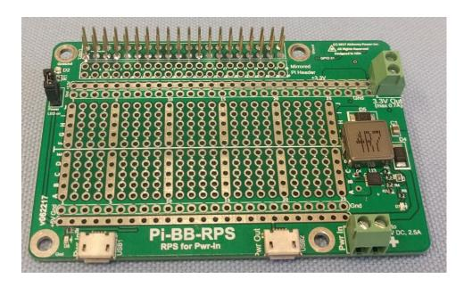
Pi-BB-RPS provides **Redundant Power Supply** capability. Second power is the micro-USB power. Power is switched seamlessly between these two sources. Priority is given to power source with higher power Voltage.
