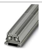
Mini feed-through terminal block, Connection method: Spring-cage connection, Cross section: 0.08 mm<sup>2</sup> - 4 mm<sup>2</sup>, AWG: 28 - 12, Width: 5.2 mm, Height: 22 mm, Color: orange, Mounting type: NS 35/7,5, NS 35/15
