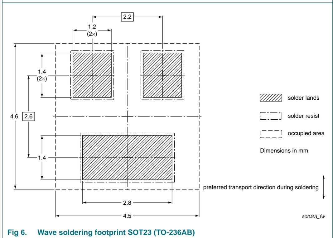
**Fig 6. Wave soldering footprint SOT23 (TO-236AB)**
