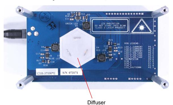
Figure 1-1. Demonstration Board, LED Side
