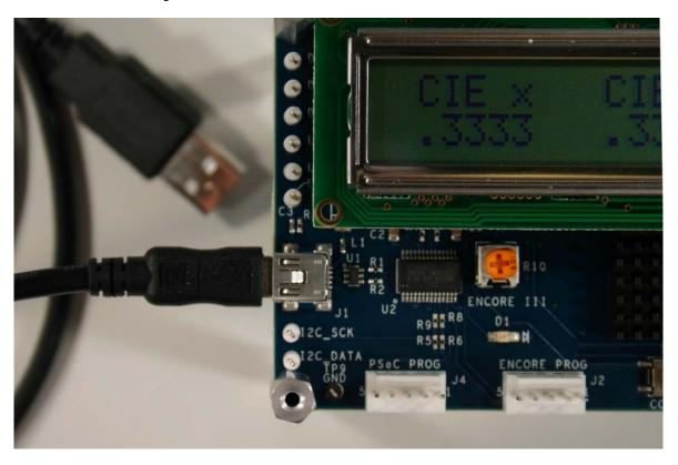
Figure 1-3. RGB Board with USB Control Cable Attached
