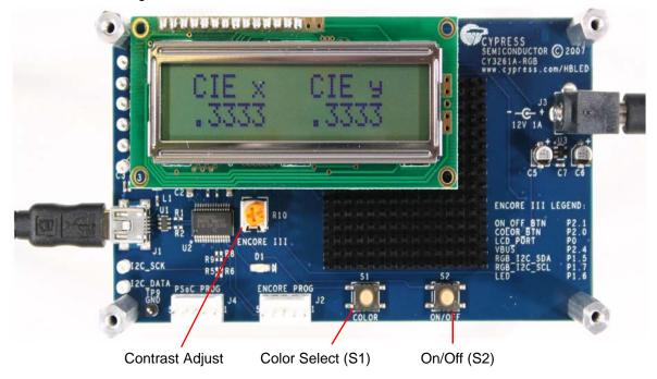
Figure 1-2. CY3261A-RGB Demonstration Board, Control Side.
