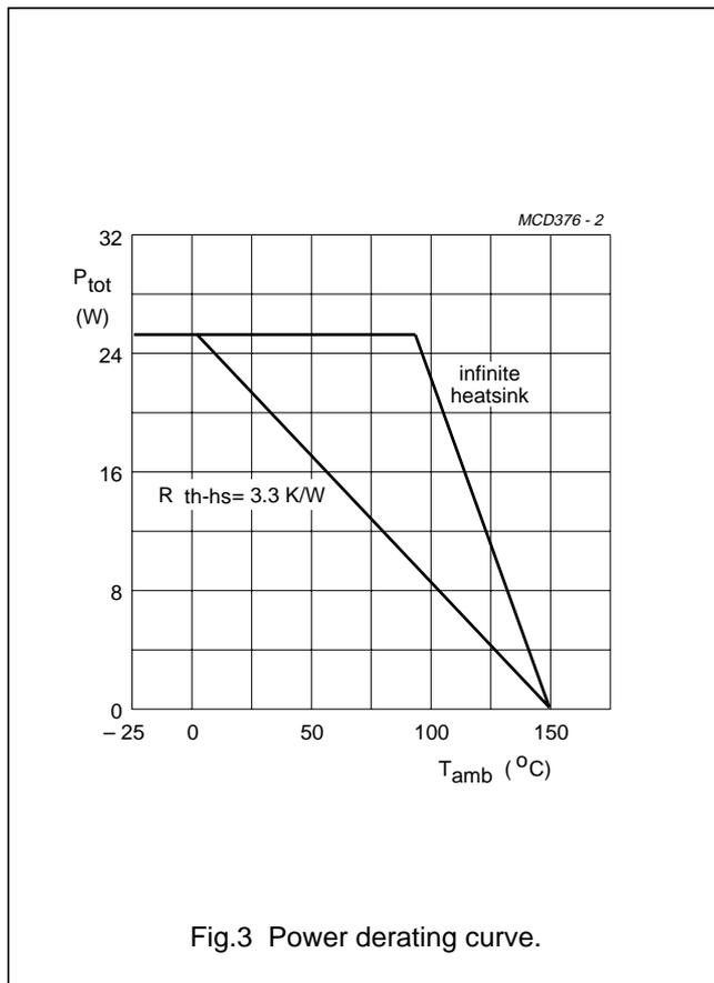
Fig.3 Power derating curve.
