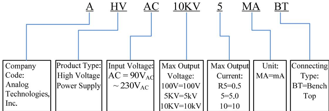
Figure 5. Naming rules of AHVAC10KV5MABT
