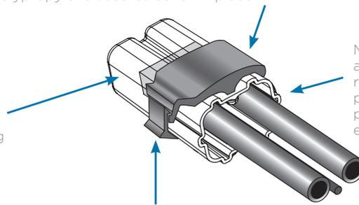
Molded cover of high abrasive and impact resistant elastomer provides rugged protection for electrical connection.
