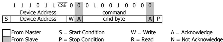
Figure 4: I<sup>2</sup>C Command to initiate a pressure conversion (OSR=4096, typ=D1)
