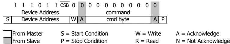
Figure 5: I<sup>2</sup>C ADC read sequence
