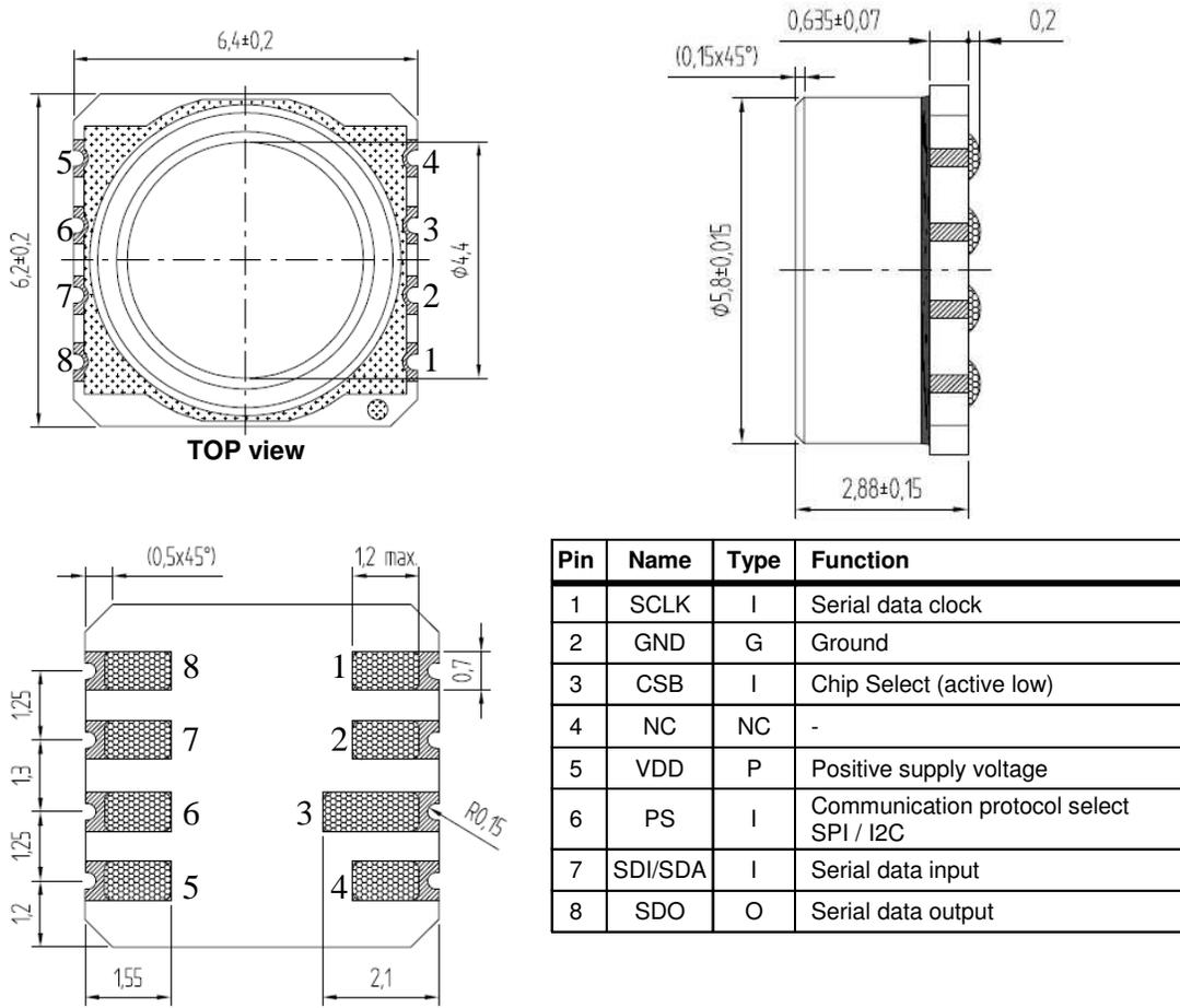
Figure 18: MS5803-14BA package outlines, pin configuration and description
