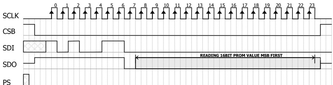
Figure 13: PROM Read sequence, address = 011 (Coefficient 3).
