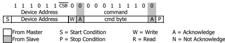
Figure 3: I<sup>2</sup>C Reset Command
