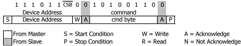
Figure 7: I<sup>2</sup>C Command to read memory address= 011 (Coefficient 3)
