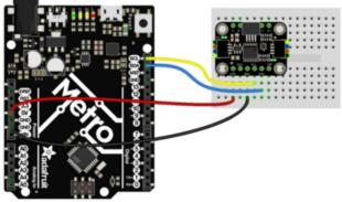
Board 5V to sensor VIN (red wire) Board GND to sensor GND (black wire) Board SCL to sensor SCL (yellow wire) Board SDA to sensor SDA (blue wire)
