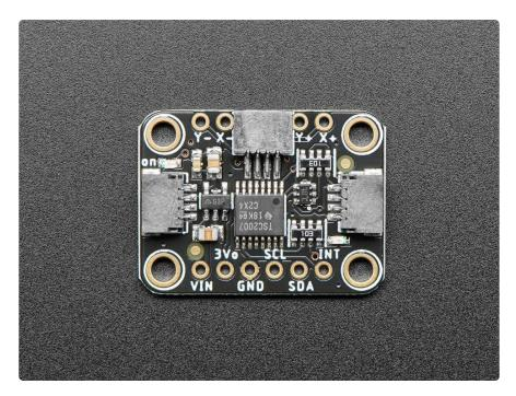
For the screens that have 1mm pitch FPC cables, you can plug the cable right into the connector. The majority of medium/large touchscreens have that kind of connector. If you have another kind of touch screen, the four X/Y contacts are available on 0.1" pitch breakouts so you can hand-solder or wire them.
