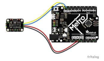
Board 5V to sensor VIN (red wire) Board GND to sensor GND (black wire) Board SCL to sensor SCL (yellow wire) Board SDA to sensor SDA (blue wire)
