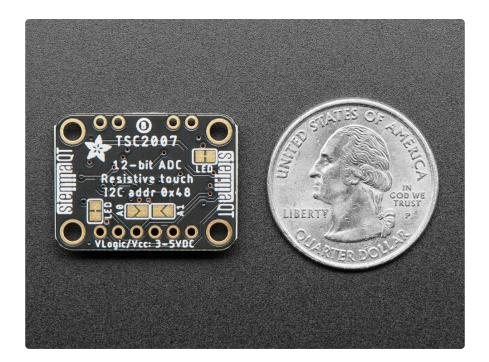
Getting started is super easy with our simple TSC2007 Arduino library () or TSC2007 CircuitPython/Python library for microcontrollers or Raspberry Pi (). Plug any 1mm-pitch 4-wire resistive touchscreen to the on-board FPC connector, then use the library example to read touch points with X, Y and Z (pressure) results returned instantaneously.
