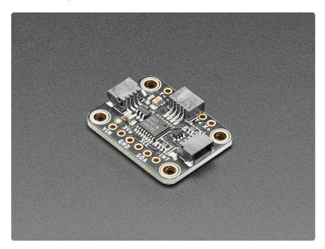
This breakout board features the TSC2007, which has an easy-to-use I2C interface. There is also an interrupt pin that you can use to indicate when a touch has been detected to your microcontroller or microcomputer.
