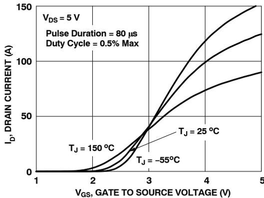
Figure 5. Transfer Characteristics
