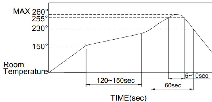
■ The condition noted above is the temperature of the copper foil on the surface of the PCB. There are cases where the temperature of the board greatly differs from the surface of the switch. Do not allow the surface temperature of the switch to exceed  $260^{\circ}\text{C}$ .
