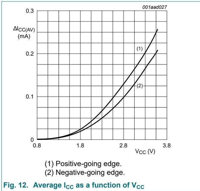
**Fig. 12. Average  $I_{\text{CC}}$  as a function of  $V_{\text{CC}}$**
