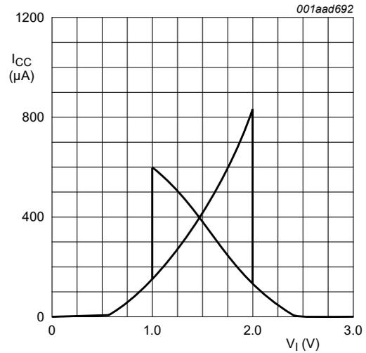
Fig. 11. Typical transfer characteristics;  $V_{CC} = 3.0\text{ V}$
