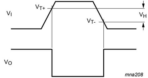
$V_{T+}$  and  $V_{T-}$  limits at 70 % and 20 %.
