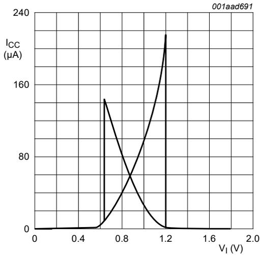
Fig. 10. Typical transfer characteristics;  $V_{CC} = 1.8\text{ V}$
