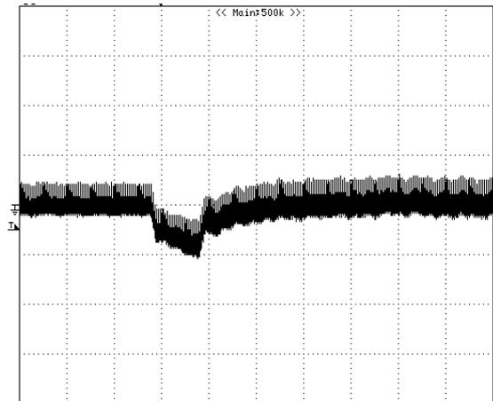
**Figure 9:** Output voltage response to step-change in load current (50%-75% of  $I_{o, \max}$ ;  $di/dt = 0.1A/\mu s$ ). Load cap:  $10\mu F$ , tantalum capacitor and  $1\mu F$  ceramic capacitor. Trace:  $V_{out}$  (20mV/div, 100us/div), Scope measurement should be made using a BNC cable (length shorter than 20 inches). Position the load between 51 mm to 76 mm (2 inches to 3 inches) from the module..
