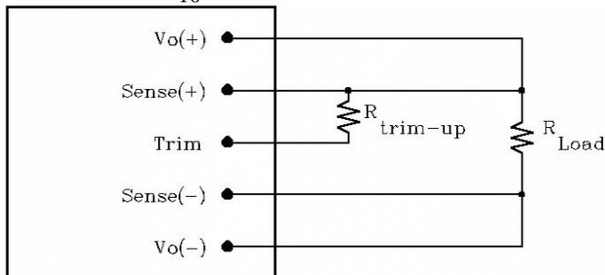
**Figure 19:** Circuit configuration for trim-up (increase output voltage)
