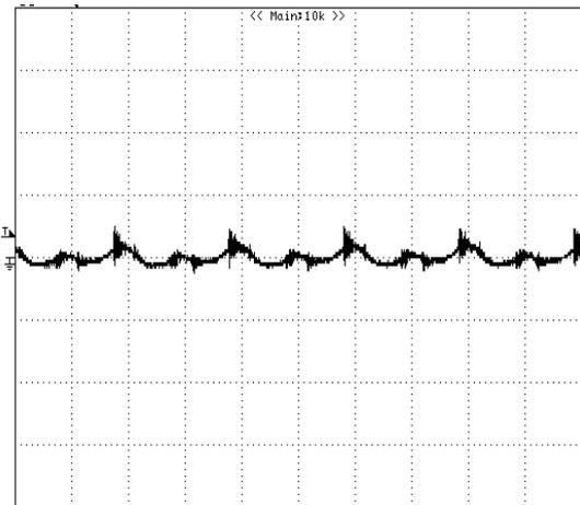
**Figure 14:** Output voltage ripple at nominal input voltage and rated load current ( $I_o=40\text{A}$ ) ( $20\text{ mV/div}$ ,  $2\mu\text{s/div}$ )
