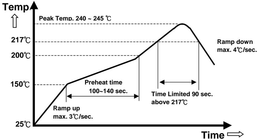
*Note: The temperature refers to the pin of E48SH, measured on the pin +Vout joint.*
