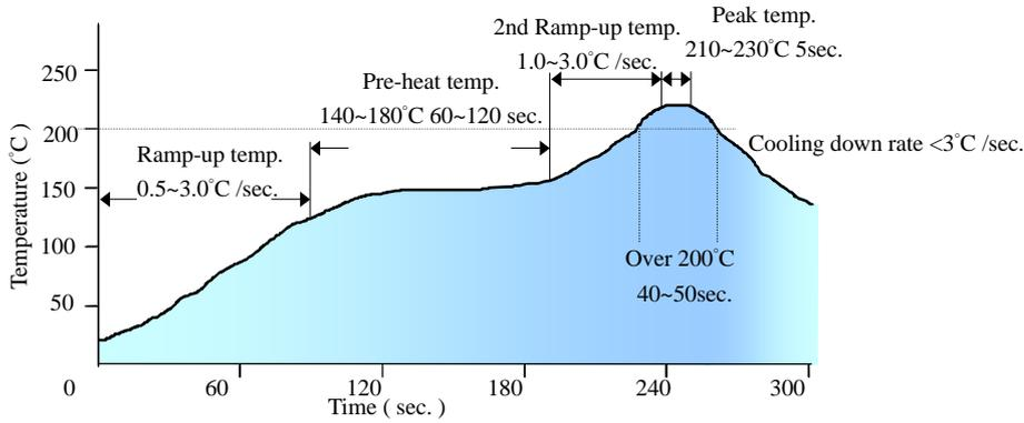
*Note: The temperature refers to the pin of E48SH, measured on the pin +Vout joint.*
