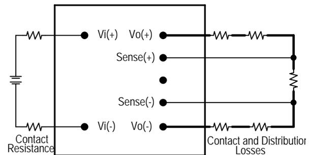
Figure 17: Effective circuit configuration for remote sense operation
