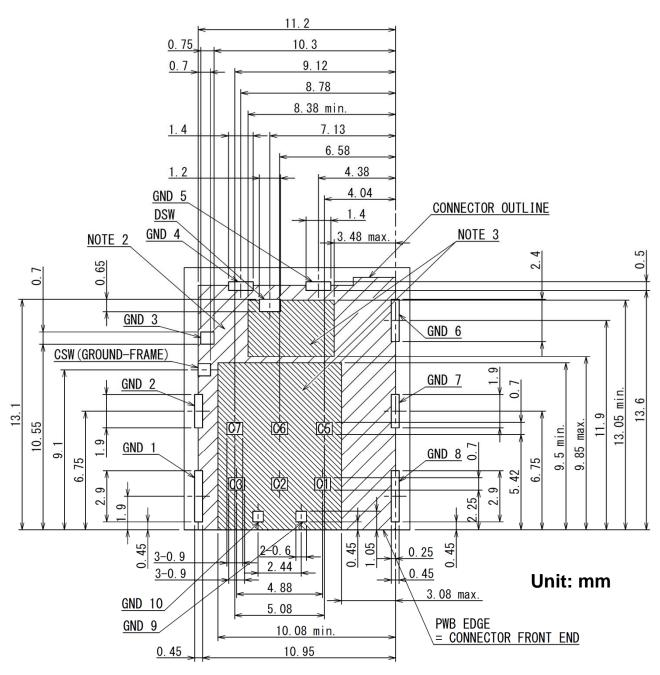
NOTE2. ONLY GND PATTERN AND VIA HOLE ALLOWED IN THIS AREA. NOTE3. NO PATTERN AND VIA HOLE IN THIS AREA.
