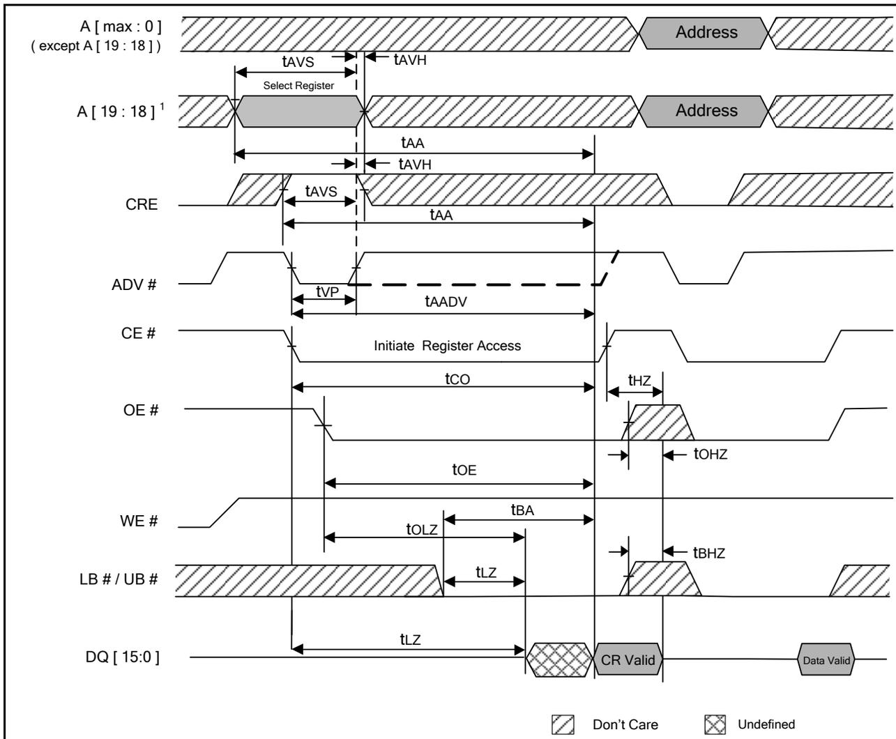
**Note:** A[19:18] = 00b to read RCR, 10b to read BCR, and 01b to read DIDR.
