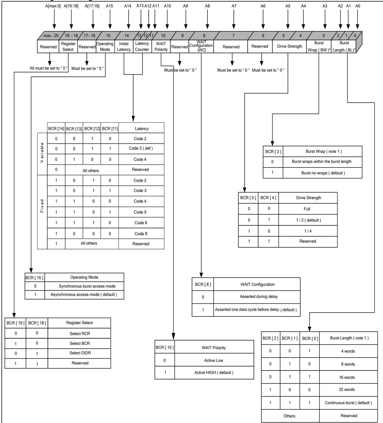
Note: 1. Burst wrap and length apply to both READ and WRITE operations.
