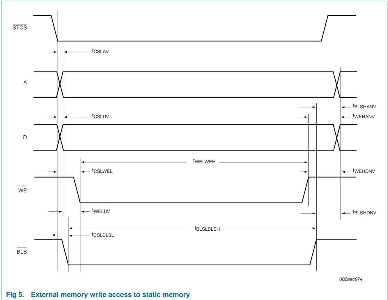
Fig 5. External memory write access to static memory
