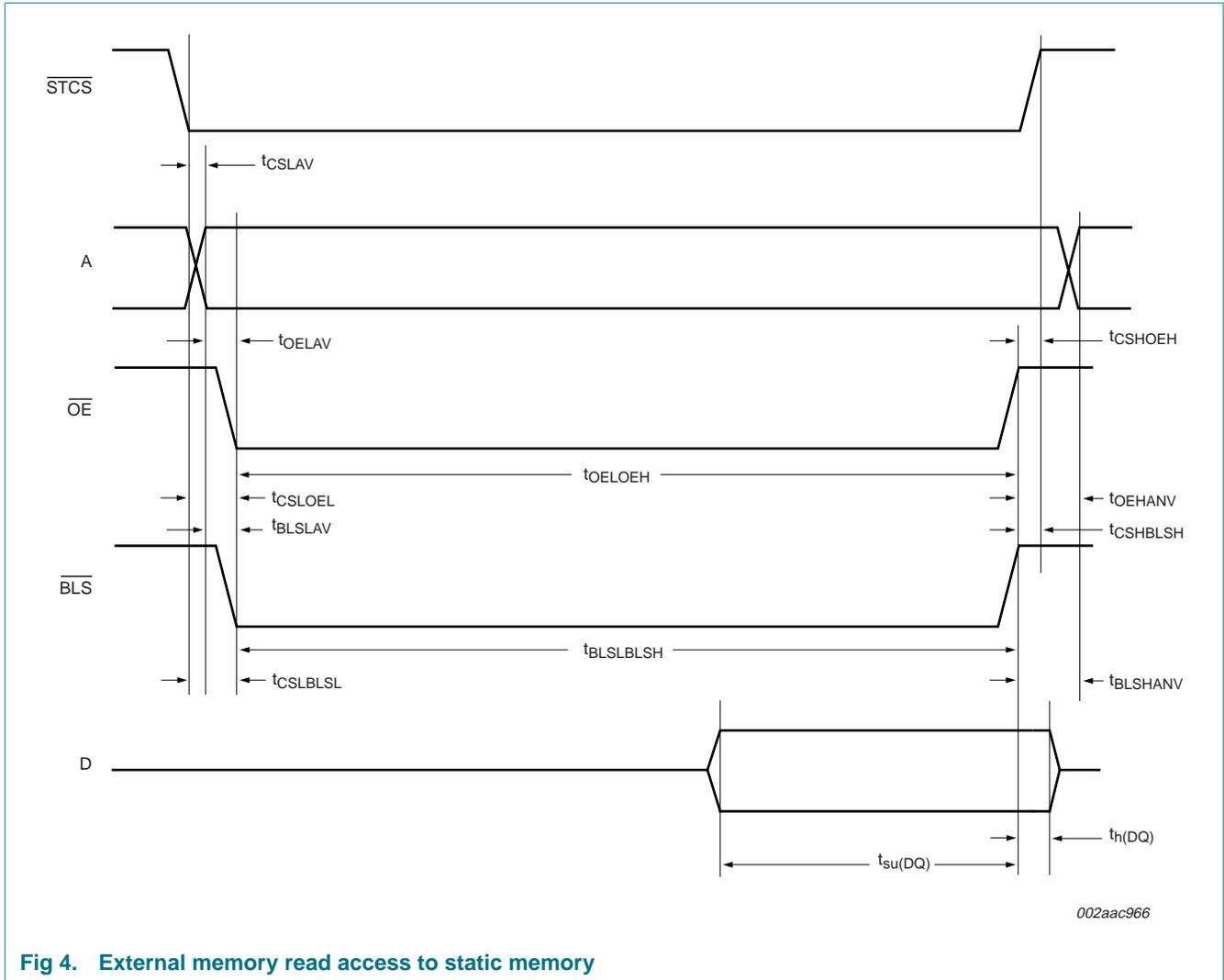
Fig 4. External memory read access to static memory
