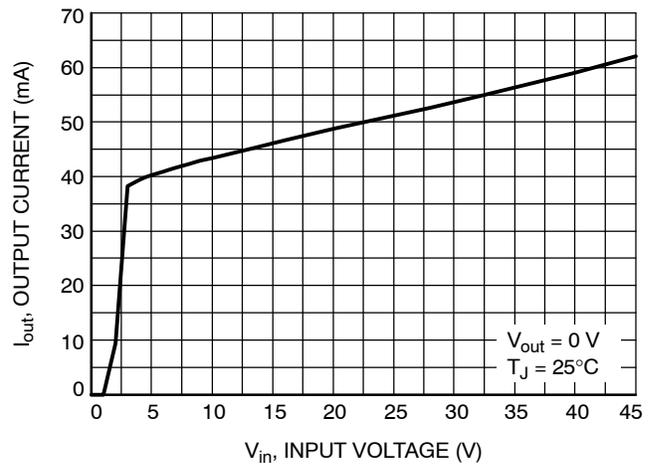
**Figure 7. Maximum Output Current vs. Input Voltage**
