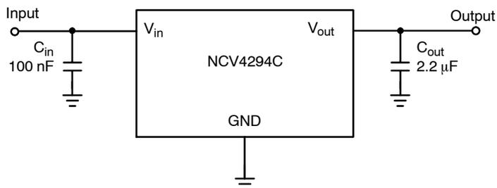
Figure 1. Applications Circuit
