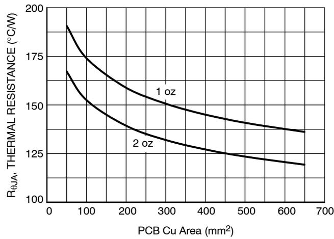
**Figure 18.  $R_{\theta JA}$  vs. PCB Cu Area**
