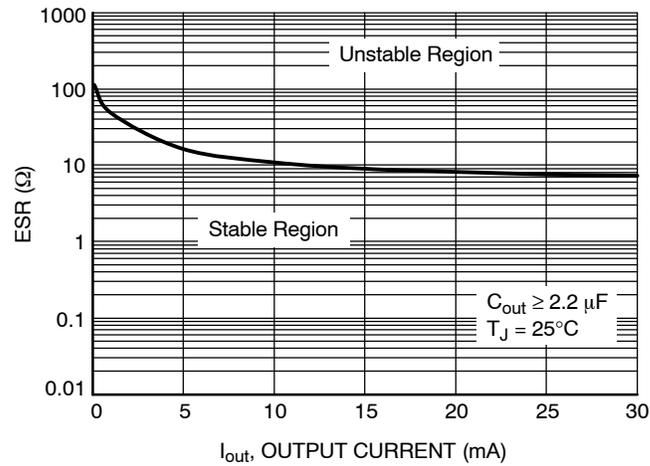
**Figure 3. Output Stability with Output Capacitor ESR**
