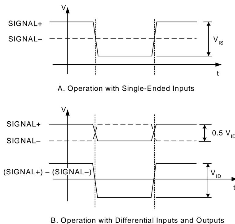
Figure 1. Differential Voltage Measurement (DIN, REFCLK, DOUT, CLKOUT)
