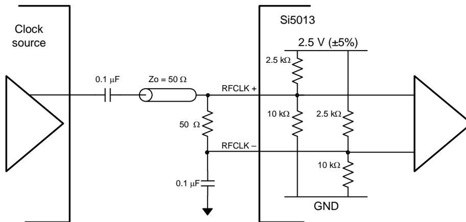
Figure 12. Single-Ended Input Termination for REFCLK (ac coupled)
