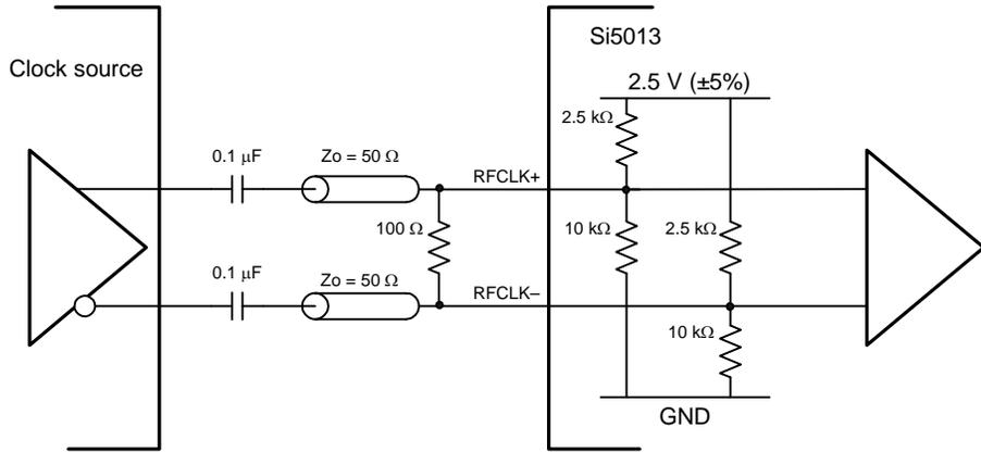
**Figure 10. Input Termination for REFCLK (ac coupled)**
