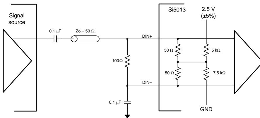
Figure 13. Single-Ended Input Termination for DIN (ac coupled)
