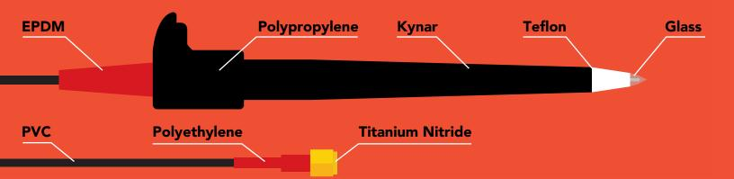
This pH probe can be fully submerged in fresh or salt water, up to the SMA connector indefinitely.
