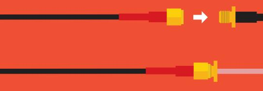
If you need to water proof a SMA connection, we highly recommend using a product like **Coax-Seal** to safely cover and prevent any water damage that may occur.
