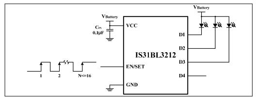
Figure 2 Application Circuit for Less Than 4 LEDs
