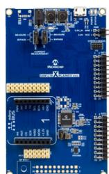
The SAM L10 Xplained Pro Evaluation Kit is ideal for evaluating and prototyping with the ultra low power SAM L10 Arm Cortex-M23 based microcontrollers.
