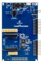
The SAM L11 Xplained Pro Evaluation Kit is ideal for evaluating and prototyping with ultra low power SAM L11 Arm Cortex-M23 based microcontrollers featuring chip-level security and Arm TrustZone Technology.
