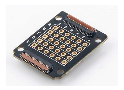
The Xadow GSM Breakout draws out 30 pins from the 35 pin Xadow connector to five rows of 0.1 spaced holes with 0.1 spacing between adjacent rows. If you solder wires or through-hole pin headers directly to the breakout pads, you can easily access: - Up to 16 General Purpose Inputs/outputs (GPIOs) - Interfaces like SPI, I2C, UART, etc. - Pinout related to peripheral devices like speaker, audio headphone and microphones
