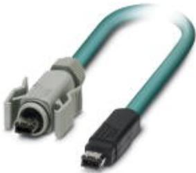
Assembled FireWire cable, shielded, color: RAL 5021 (water blue), PUR outer sheath, FireWire/IP67 on FireWire/standard, length: 2 m
