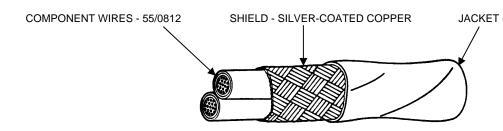
JACKET - LOW OUTGASSING, RADIATION-CROSSLINKED, MODIFIED ETFE
