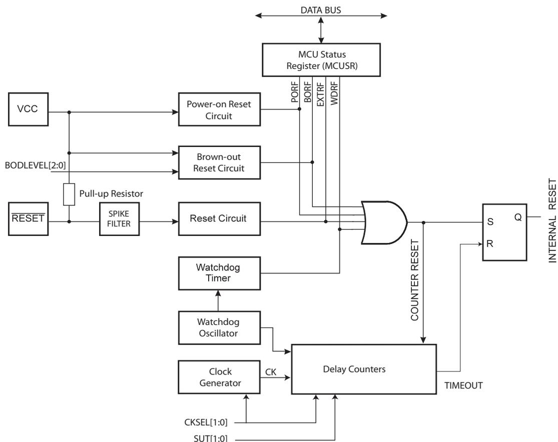
The I/O ports of the AVR are immediately reset to their initial state when a reset source goes active. This does not require any clock source to be running.
