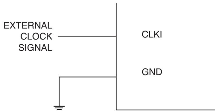
When this clock source is selected, start-up times are determined by SUT Fuses as shown in [Table 6-3](#).
