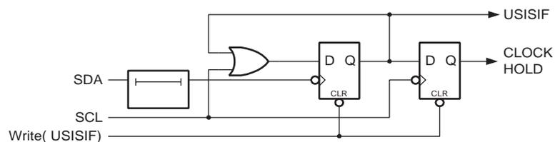
The start condition detector works asynchronously and can therefore wake up the processor from power-down sleep mode. However, the protocol used might have restrictions on the SCL hold time. Therefore, when using this feature the oscillator start-up time (set by CKSEL fuses, see [“Clock Sources” on page 24](#)) must also be taken into consideration. Refer to the description of the USISIF bit on [page 114](#) for further details.
