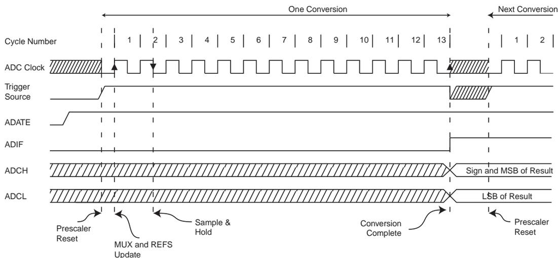
In Free Running mode, a new conversion will be started immediately after the conversion completes, while ADSC remains high. See [Figure 16-7](#).
