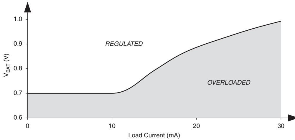
**Figure 20-4.** Typical Transition Range Between Modes of Operation
