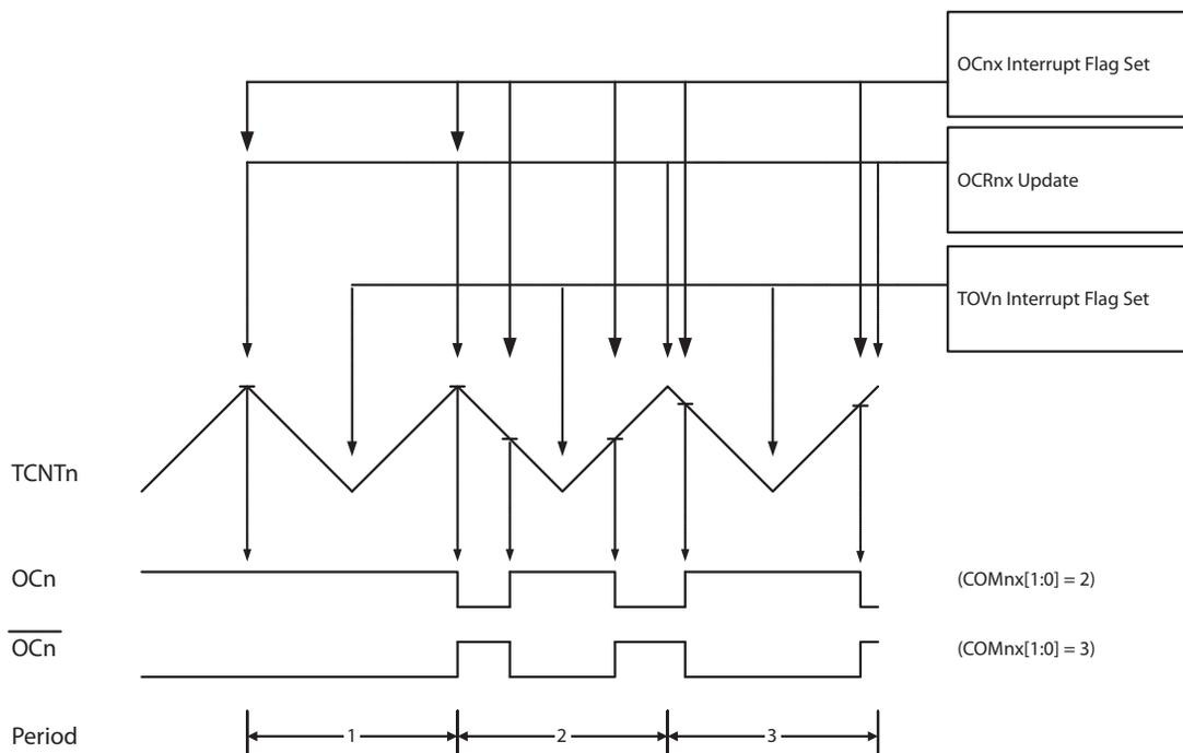
The Timer/Counter Overflow Flag (TOVn) is set each time the counter reaches BOTTOM. The Interrupt Flag can be used to generate an interrupt each time the counter reaches the BOTTOM value.
