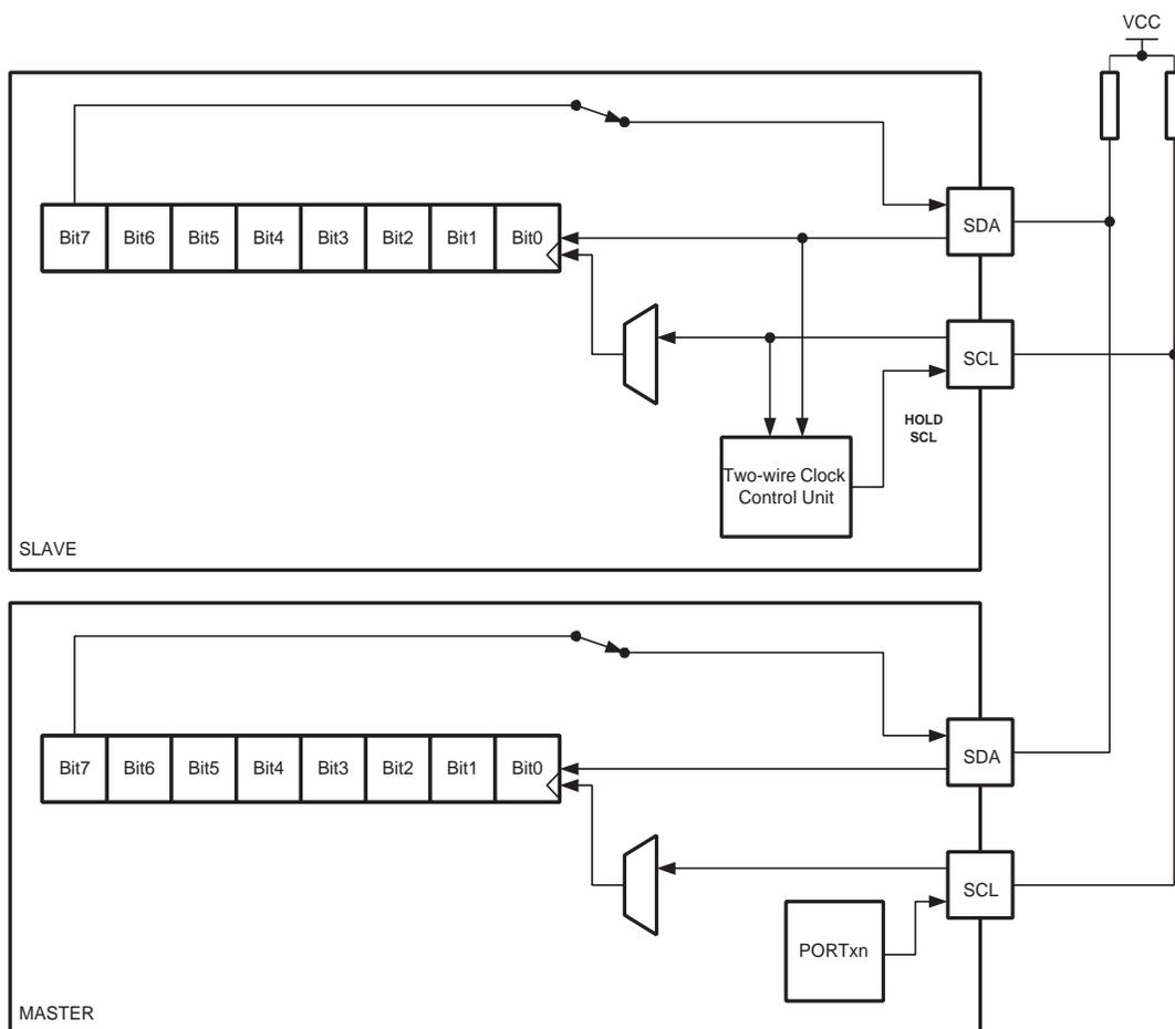
The data direction is not given by the physical layer. A protocol, like the one used by the TWI-bus, must be implemented to control the data flow.
