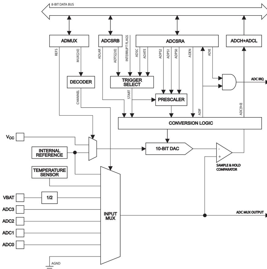
The ADC contains a Sample and Hold circuit which ensures that the input voltage to the ADC is held at a constant level during conversion.
