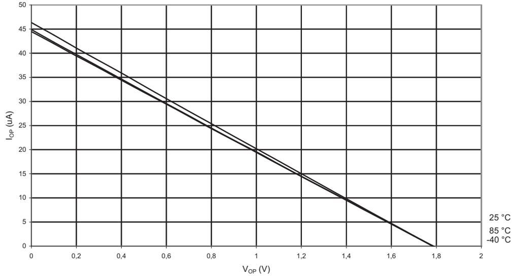
**Figure 21-20.** Pull-up Resistor Current vs. Input Voltage (I/O Pin,  $V_{CC} = 2.7V$ )
