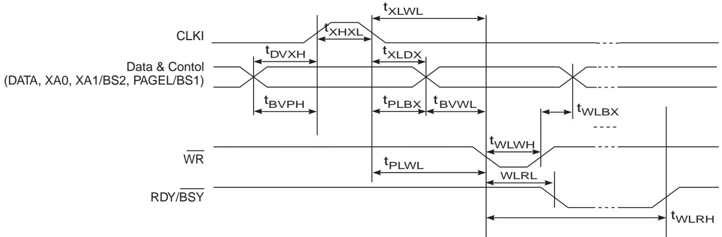
Note: The timing requirements in Figure 20-5 (i.e.,  $t_{DVXH}$ ,  $t_{XHXL}$ , and  $t_{XLDX}$ ) also apply to reading operation.
