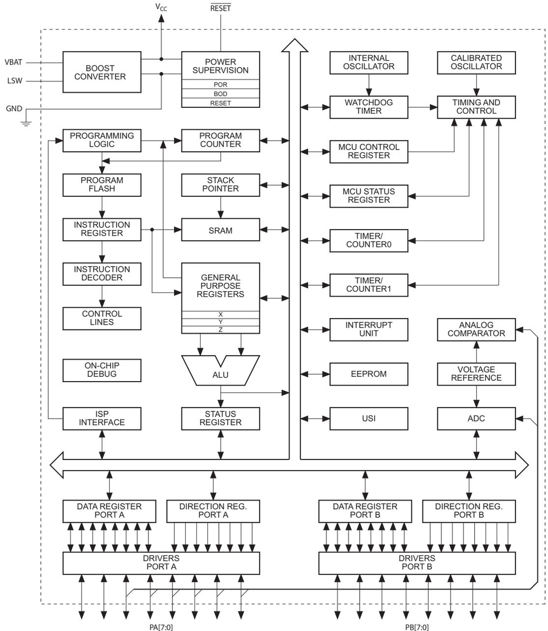
The AVR core combines a rich instruction set with 32 general purpose working registers. All the 32 registers are directly connected to the Arithmetic Logic Unit (ALU), allowing two independent registers to be accessed in one single instruction executed in one clock cycle. The resulting
