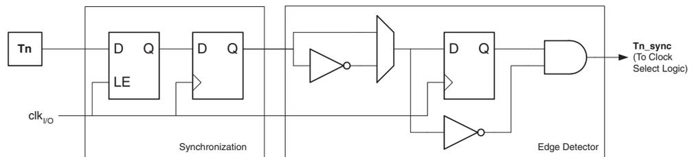
The synchronization and edge detector logic introduces a delay of 2.5 to 3.5 system clock cycles from an edge has been applied to the  $T_n$  pin to the counter is updated.
