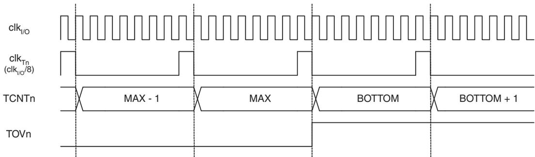
[Figure 12-10 on page 91](#) shows the setting of OCFnB in all modes and OCFnA in all modes except CTC mode and PWM mode, where OCRnA is TOP.
