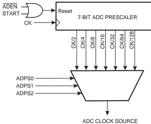
When initiating a single ended conversion by setting the ADSC bit in ADCSRA, the conversion starts at the following rising edge of the ADC clock cycle.
