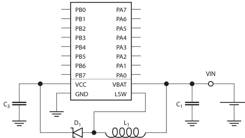
When the boost converter is not connected the microcontroller can be powered directly from an external source and is then subject to the standard supply voltage limits defined in “[Electrical Characteristics](#)” on page 158.
