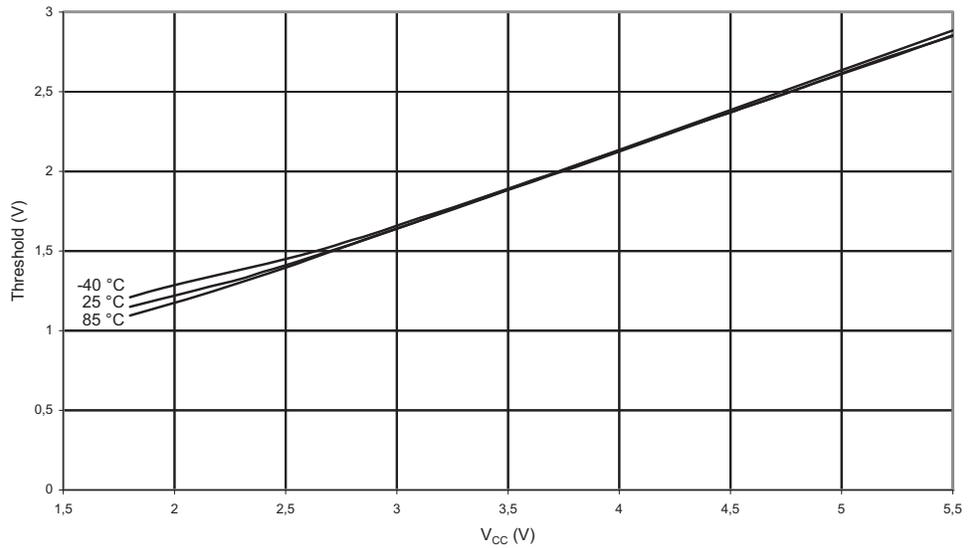
**Figure 21-37.**  $V_{IL}$ : Input Threshold Voltage vs.  $V_{CC}$  (Reset Pin as I/O, Read as '0')
