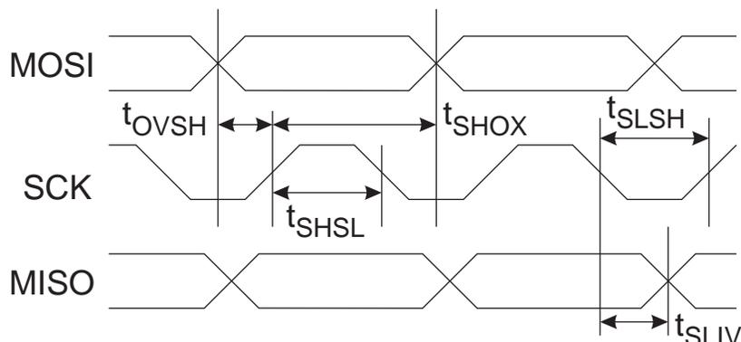
**Figure 20-9.** Serial Programming Waveforms
