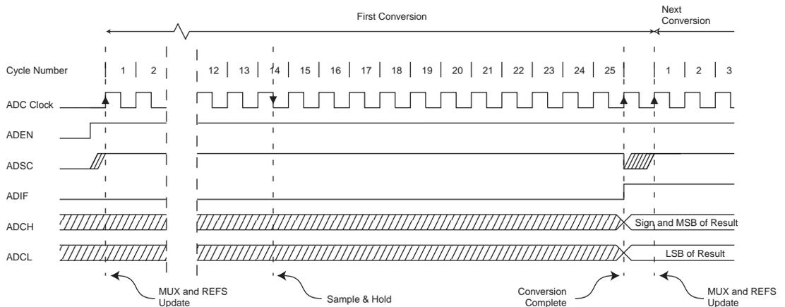
The actual sample-and-hold takes place 1.5 ADC clock cycles after the start of a normal conversion and 13.5 ADC clock cycles after the start of a first conversion. See [Figure 16-5](#). When a conversion is complete, the result is written to the ADC Data Registers, and ADIF is set. In Single Conversion mode, ADSC is cleared simultaneously. The software may then set ADSC again, and a new conversion will be initiated on the first rising ADC clock edge.
