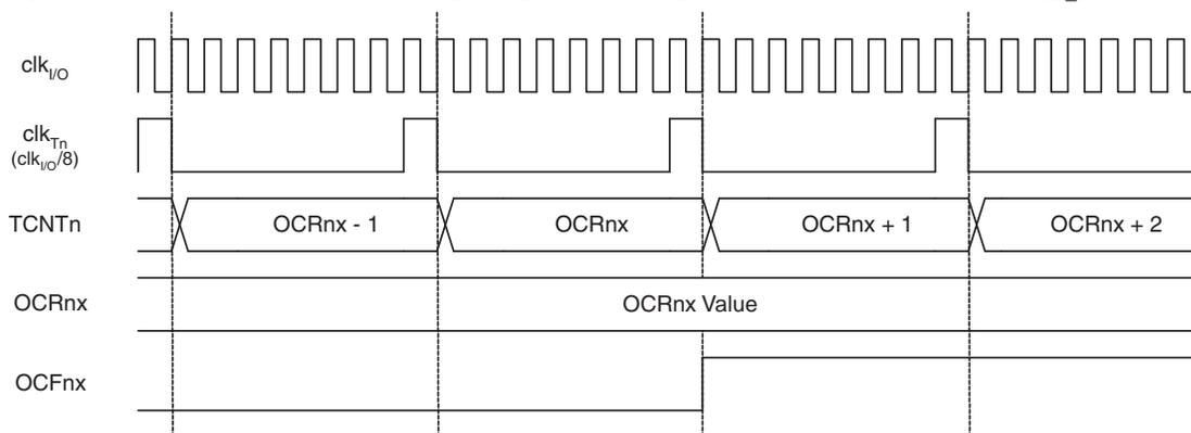
Figure 12-11 on page 91 shows the setting of OCFnA and the clearing of TCNTn in CTC mode and fast PWM mode where OCRnA is TOP.
