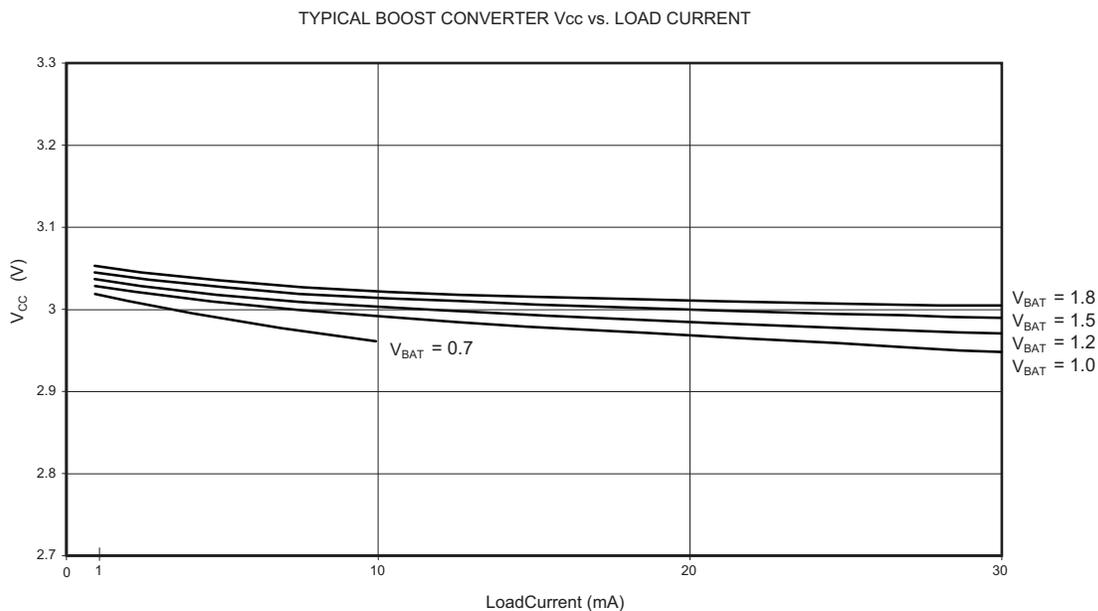
**Figure 21-2.** Boost Converter Efficiency vs. Load Current and  $V_{BAT}$  Voltage
