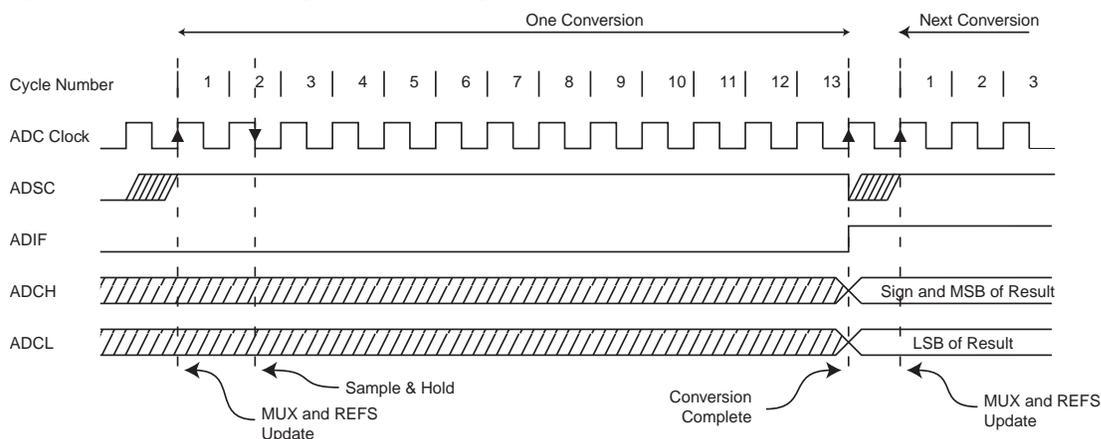
When Auto Triggering is used, the prescaler is reset when the trigger event occurs, as shown in [Figure 16-6](#) below. This assures a fixed delay from the trigger event to the start of conversion. In this mode, the sample-and-hold takes place two ADC clock cycles after the rising edge on the trigger source signal. Three additional CPU clock cycles are used for synchronization logic.
