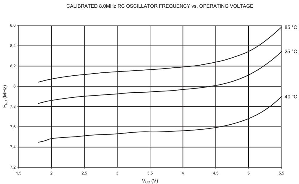
**Figure 21-51.** Frequency of Calibrated 8 MHz RC Oscillator vs. Temperature
