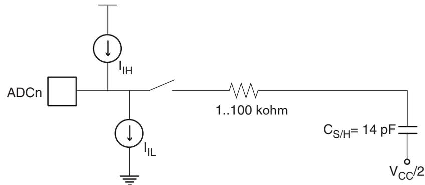
Note: The capacitor in the figure depicts the total capacitance, including the sample/hold capacitor and any stray or parasitic capacitance inside the device. The value given is worst case.
