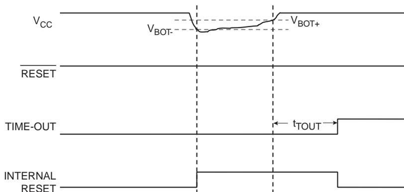
It is recommended to use only the lowest BOD level (1.8V), when using the integrated boost converter. See [“Power Supply and On-Chip Boost Converter” on page 35](#).
