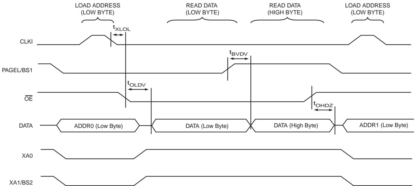
**Figure 20-7.** Parallel Programming Timing, Loading Sequence with Timing Requirements
