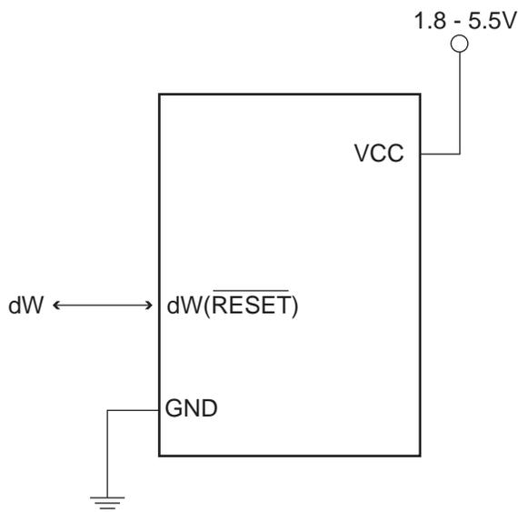
Figure 17-1 shows the schematic of a target MCU, with debugWIRE enabled, and the emulator connector. The system clock is not affected by debugWIRE and will always be the clock source selected by the CKSEL Fuses.
