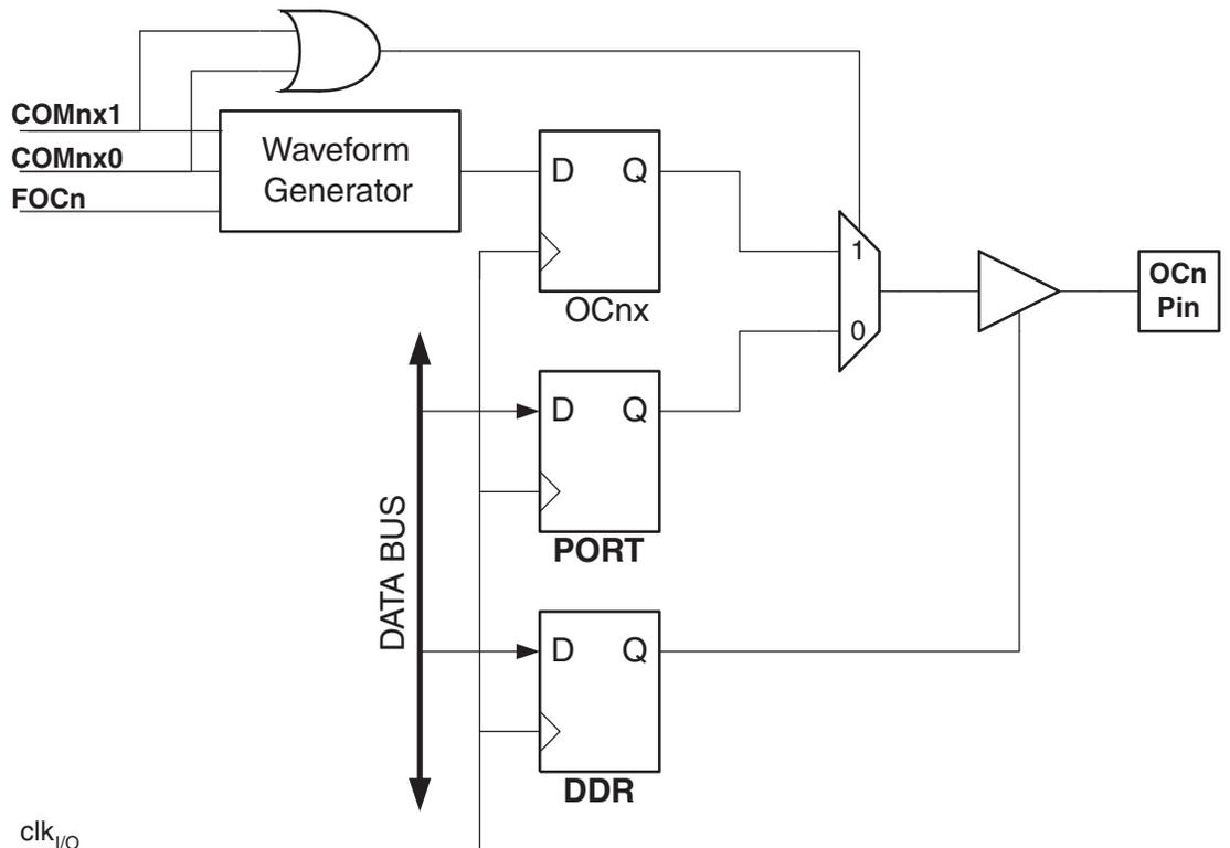
The general I/O port function is overridden by the Output Compare (OC<sub>n</sub>) from the Waveform Generator if either of the COM<sub>n</sub>[1:0] bits are set. However, the OC<sub>n</sub> pin direction (input or output) is still controlled by the Data Direction Register (DDR) for the port pin. The Data Direction
