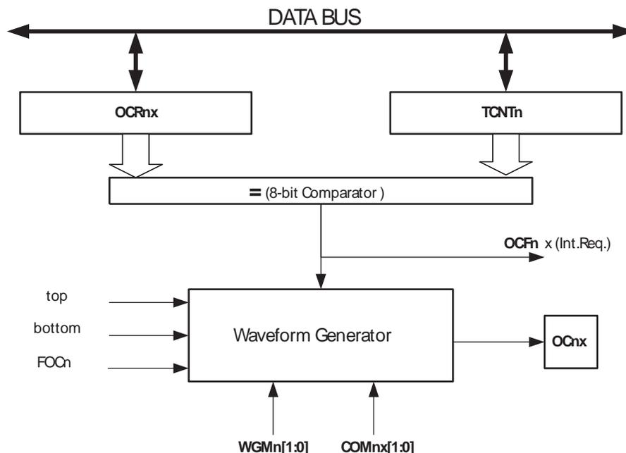
The OCRnx Registers are double buffered when using any of the Pulse Width Modulation (PWM) modes. For the normal and Clear Timer on Compare (CTC) modes of operation, the double buffering is disabled. The double buffering synchronizes the update of the OCRnx Compare Registers to either top or bottom of the counting sequence. The synchronization prevents the occurrence of odd-length, non-symmetrical PWM pulses, thereby making the output glitch-free.
