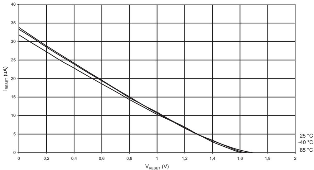
**Figure 21-23.** Reset Pull-up Resistor Current vs. Reset Pin Voltage ( $V_{CC} = 2.7V$ )
