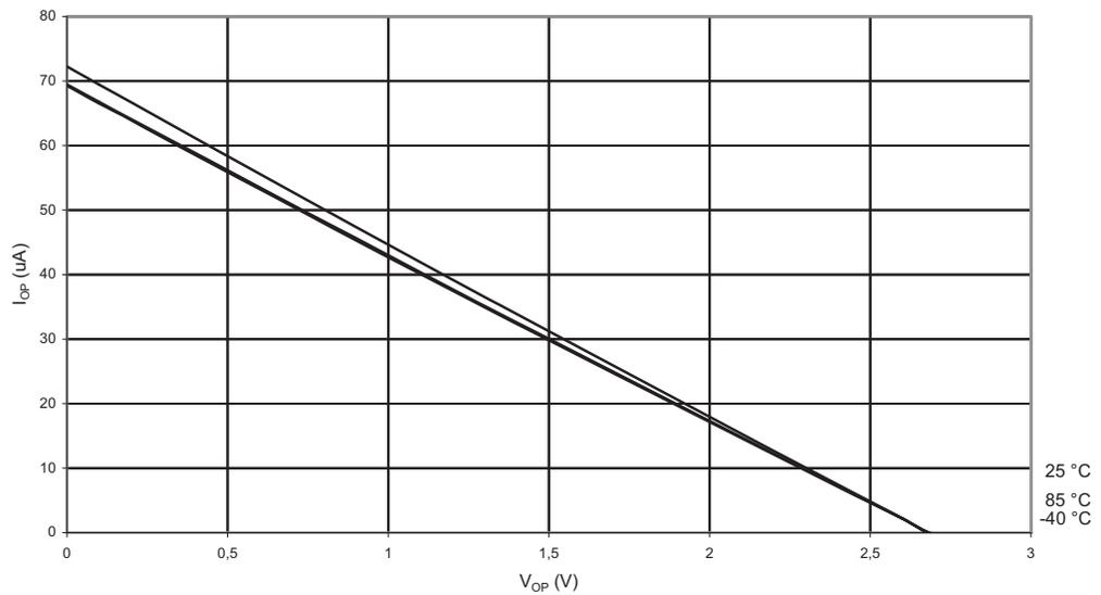
**Figure 21-21.** Pull-up Resistor Current vs. Input Voltage (I/O Pin,  $V_{CC} = 5V$ )
