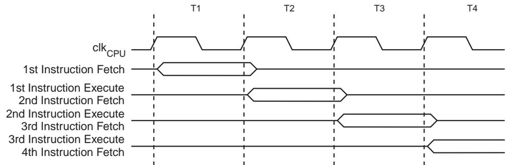
Figure 4-5 on page 12 shows the internal timing concept for the Register File. In a single clock cycle an ALU operation using two register operands is executed, and the result is stored back to the destination register.
