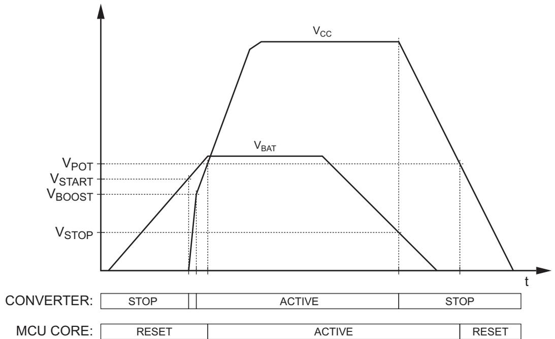
When input voltage  $V_{BAT}$  falls below  $V_{STOP}$  the converter enters Stop Mode and output voltage  $V_{CC}$  begins to fall. When converter output voltage, i.e. the supply voltage of the microcontroller, falls below  $V_{POT}$  the MCU will go into reset.
