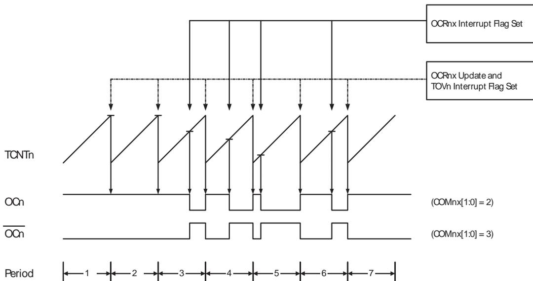
The Timer/Counter Overflow Flag (TOVn) is set each time the counter reaches TOP. If the interrupt is enabled, the interrupt handler routine can be used for updating the compare value.
