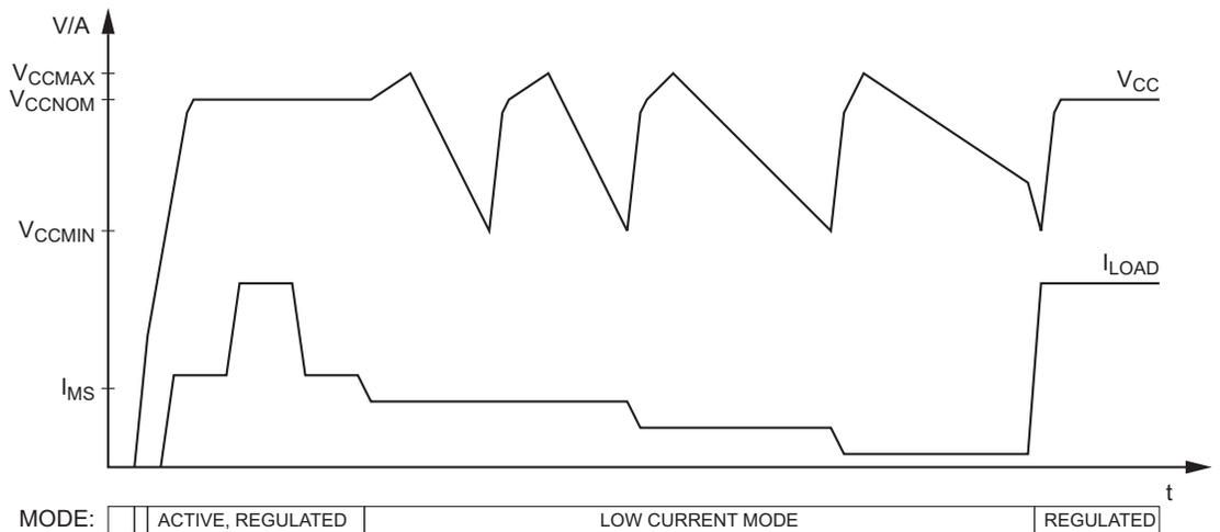
Note: The figure is not to scale. Typically, the switching time (rising voltage) is measured in hundreds of microseconds and idle time (falling voltage) is measured in seconds.
