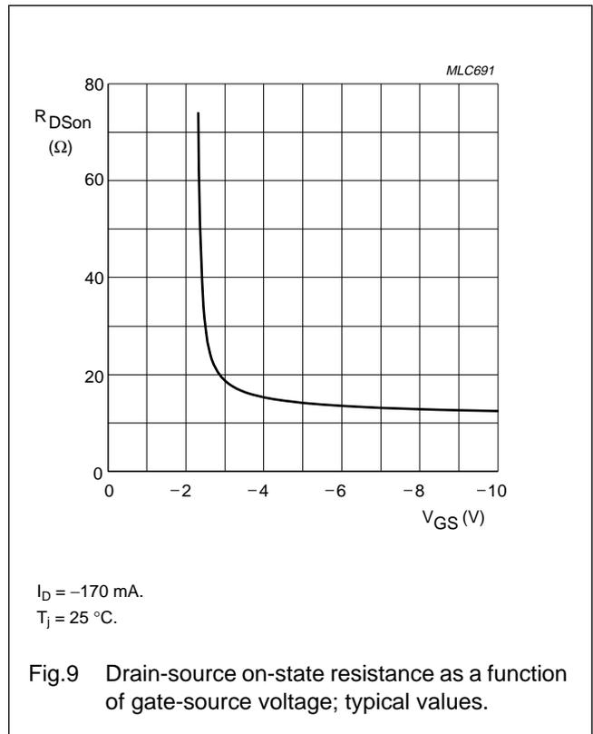
P-channel enhancement mode vertical D-MOS transistors
