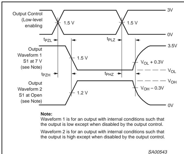
Waveform 2. 3-State Output Enable and Disable Times
