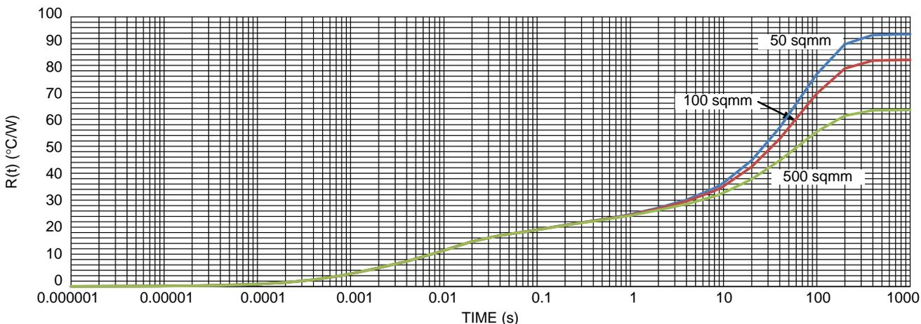
Figure 15. SOIC 28-Lead Single Pulse Heating Curve
