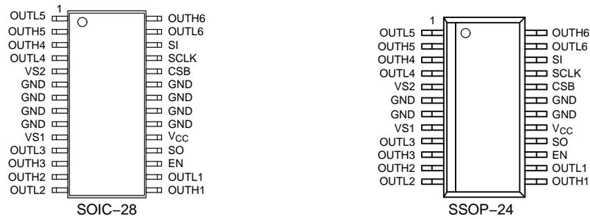
Figure 2. Pin Connection
