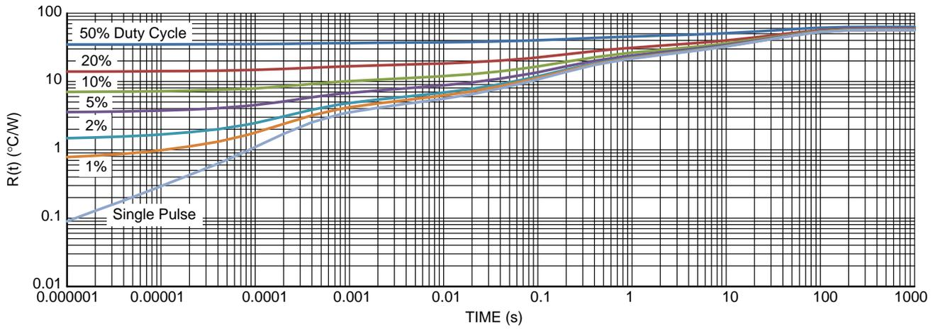
Figure 18. SSOP24 Lead Single Pulse Heating Curve
