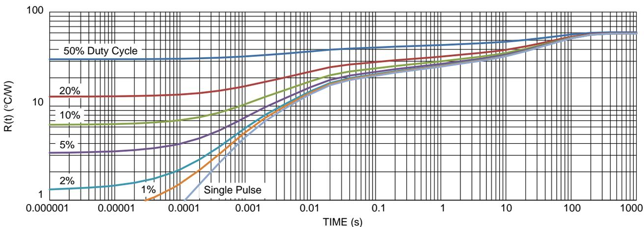
Figure 16. SOIC 28-Lead Thermal Duty Cycle Curve on 986 mm<sup>2</sup> Spreader Test Board
