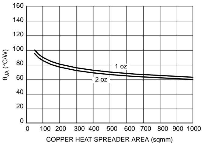
Figure 13. SOIC-28  $\theta_{JA}$  vs. Copper Spreader Area
