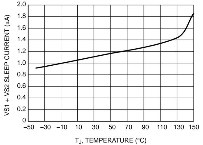
Figure 12. VS1 + VS2 Sleep Current vs. Temperature
