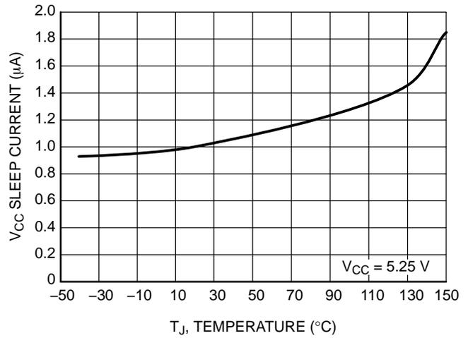
Figure 10. V<sub>CC</sub> Sleep Supply Current vs. Temperature
